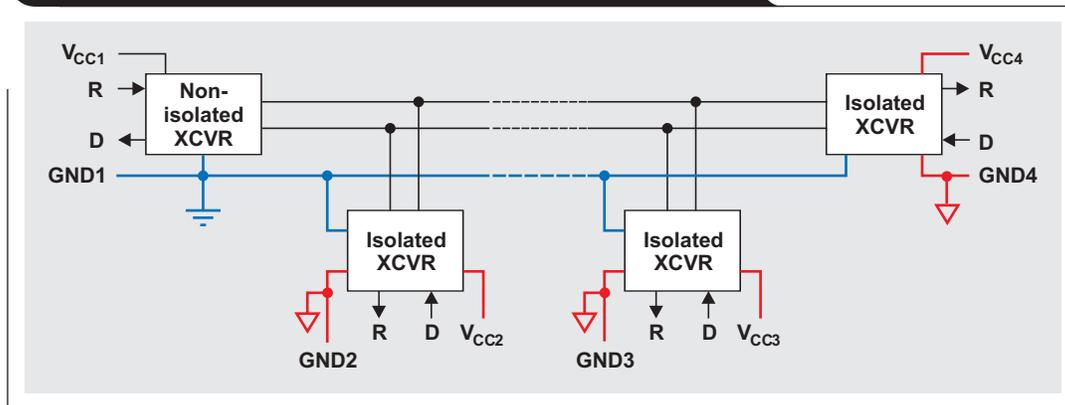
While Figure 8 shows the detailed connection of two remote transceiver nodes, Figure 9 shows an example of an isolated data-transmission system using multiple transceivers. Here all but one transceiver connect to the bus via isolation. The non-isolated transceiver on the left provides the single-ground reference for the entire bus.
