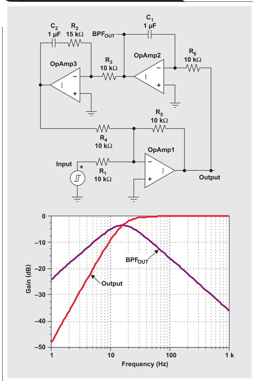
advantage it would have over any other common topology is that it can implement an HPF with no capacitors in the forward signal path.
