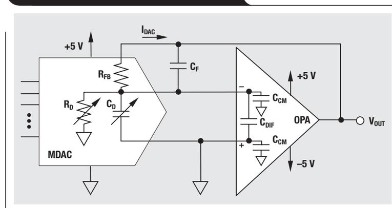
the operational amplifier, as well as the input-differential capacitance ( $C_{DIF}$ ) and common-mode capacitance ( $C_{CM}$ ), directly affect the stability of this circuit.
