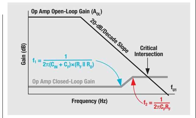
Figure 2c. Model’s frequency response with a low-bandwidth amplifier
