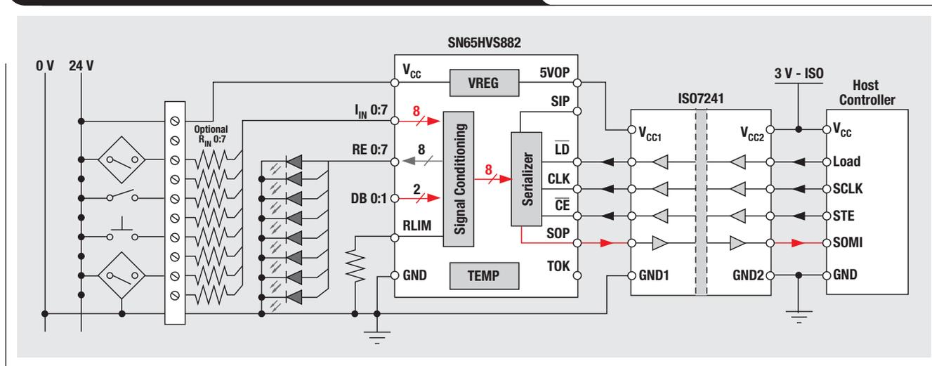
The designer can further reduce the number of external components by using the integrated debounce filter, set to filter pulses of less than 3 ms or 1 ms in duration. For the fastest acquisition of glitch-free switches, bypass the filter as well.
