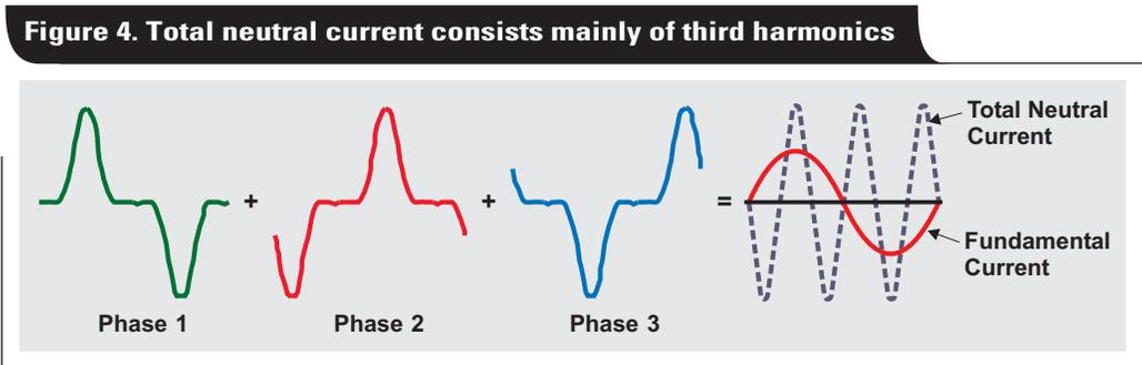
While the third and fifth harmonics of the fundamental 60-Hz line frequency make up the lion's share of the harmonic content, the vector sum of all frequency components (including the 60-Hz fundamental) can reach peak values that exceed the amplitude of the fundamental phase current by more than 100%.
