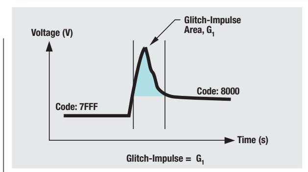
switching from 7FFFh to 8000h (for a 16-bit DAC). The R-2R back-DAC, like the MDAC, typically has excellent low noise, INL, and DNL performance, with medium settling-time capability.
