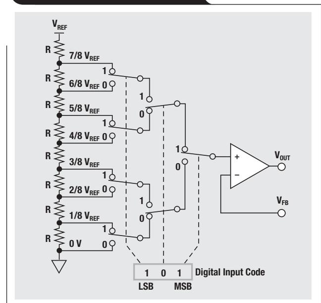
with good DNL performance across the entire input code range. The glitch energy is typically lower than other types of DACs; however, the INL performance is generally larger and dependent on resistive, on-chip matching. On the other hand, a DAC in a control loop lessens the impact of high linearity. The noise of string DACs is also relatively high because of the resistive string-array impedance.
