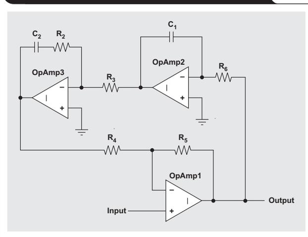
Figure 7. Inverting amplifier with feedback to non-inverting terminal
