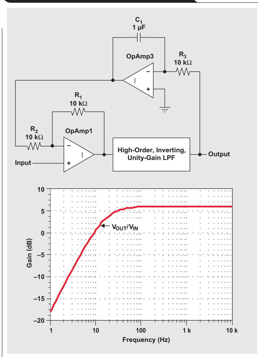
$$f = \frac{\frac{R_1}{R_2} G_{LPF}}{2\pi R_3 C_1}. \quad (2)$$
