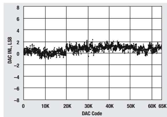
next, as may be with R-2R architectures, this technique may prove to be counterproductive instead of an improvement in DAC performance. The string DAC topology is best suited for this calibration technique because it is inherently monotonic (a requirement for this technique) and jumps from one code to the next are relatively small as compared to other DAC topologies.
