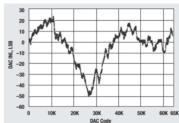
Figure 6b. A correction step of 64 LSB (1024 out of the 65,536 points) reduces the INL error to less than  $\pm 3$  LSB
