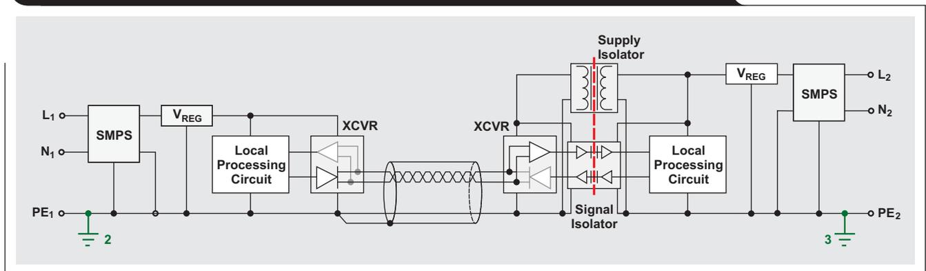
**Figure 9. Isolation of multiple fieldbus-transceiver stations**
