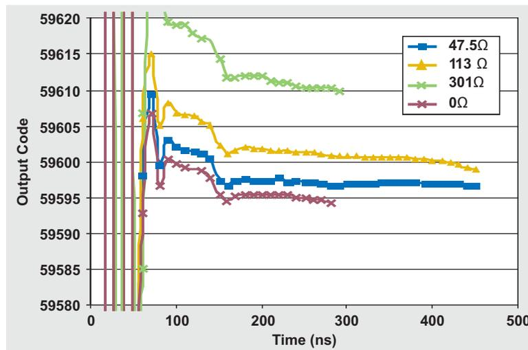
**Figure 7. Effects of Changing Feedback Resistors**
