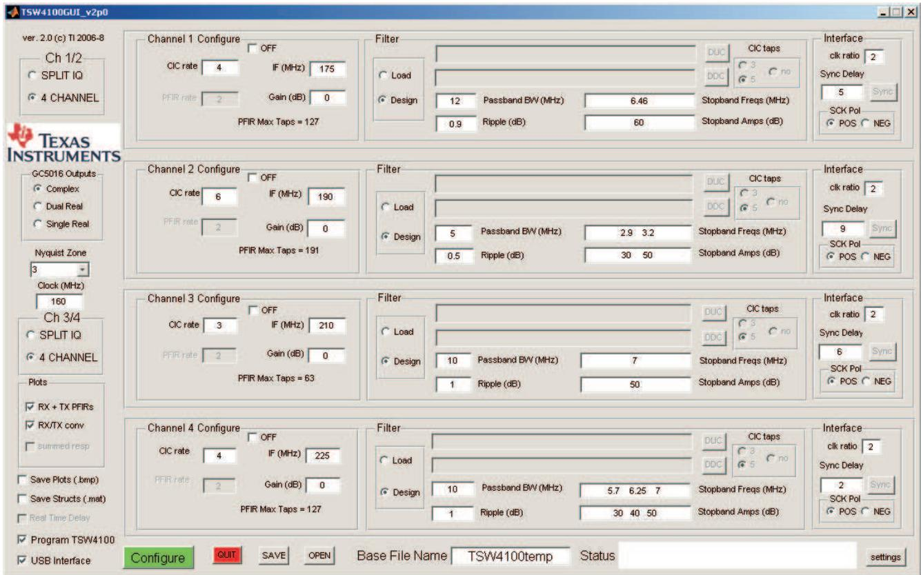
Figure 68. TSW4100GUI Settings to Generate Third Nyquist Zone
