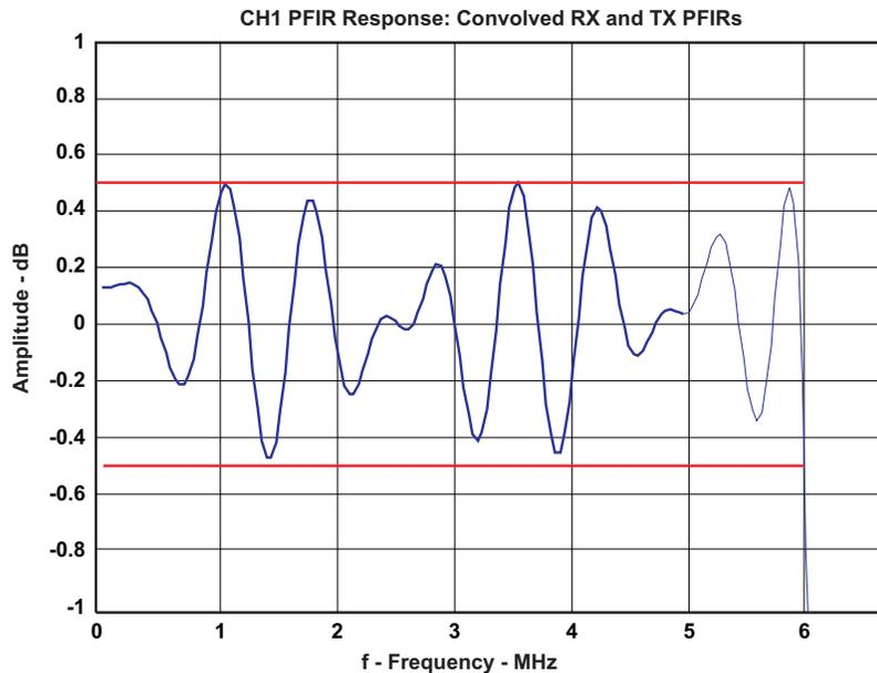
Figure 38. Passband for the Composite Frequency Response
