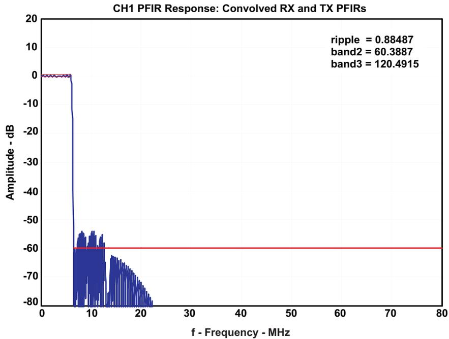
Figure 47. Complete Response of Successful Filter Design
