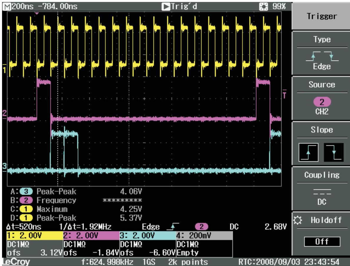
Figure 60. Channel 3 Interface Timing With a Sync Delay of 129
