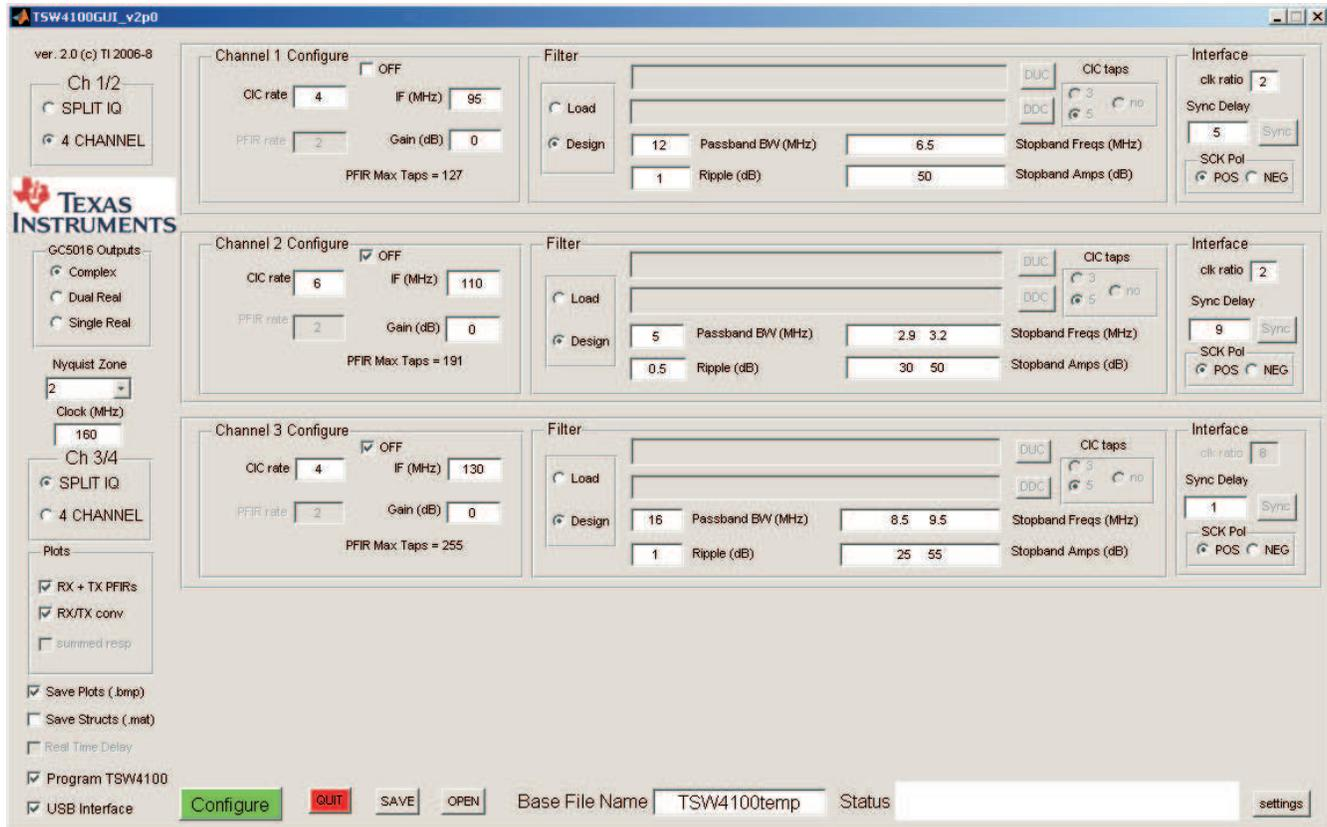
Figure 51. TSW4100 Interface with Filter Design Settings
