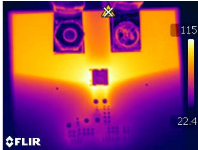
Figure 6-1. Thermal Image of the AMC-AMP-200APK-EVM
