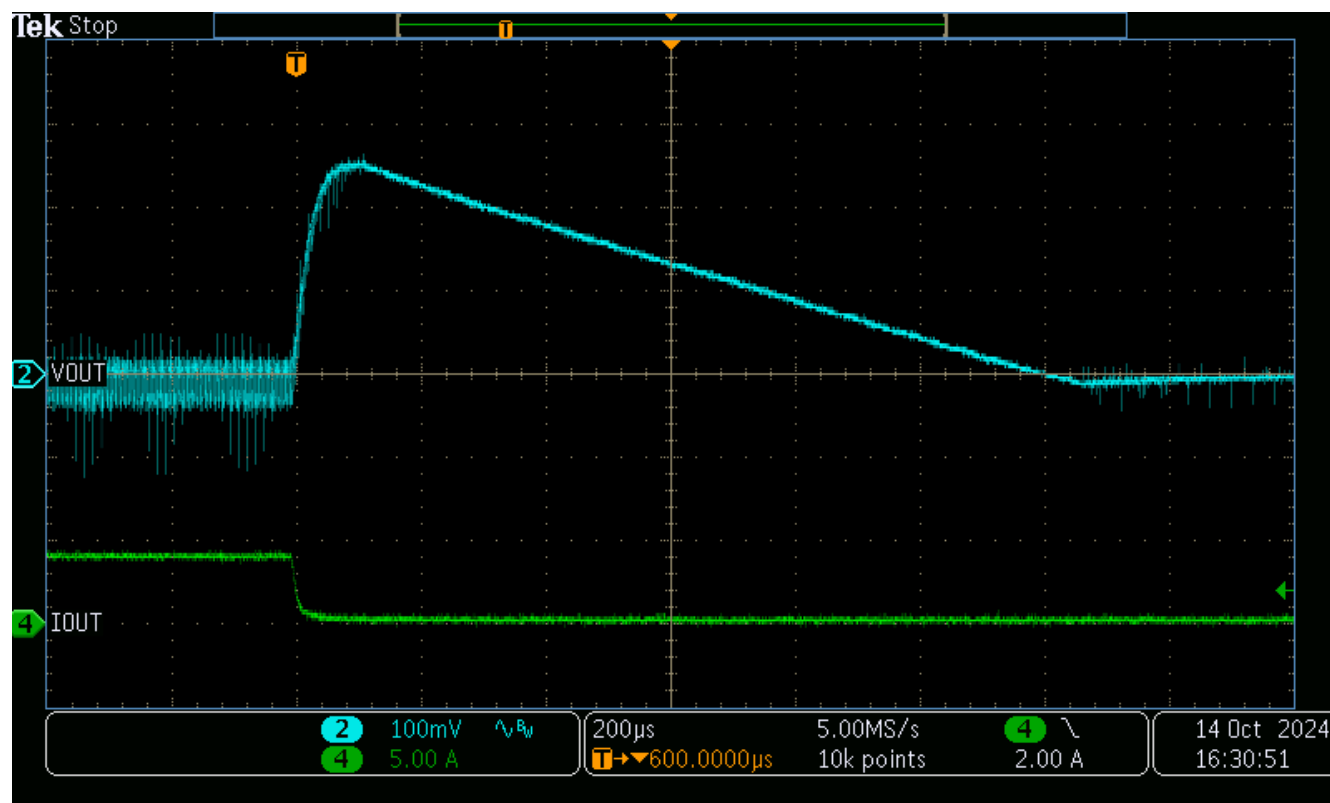
Figure 3-3. Transient Response to Load Step 4A to 100mA at 8A/μs
