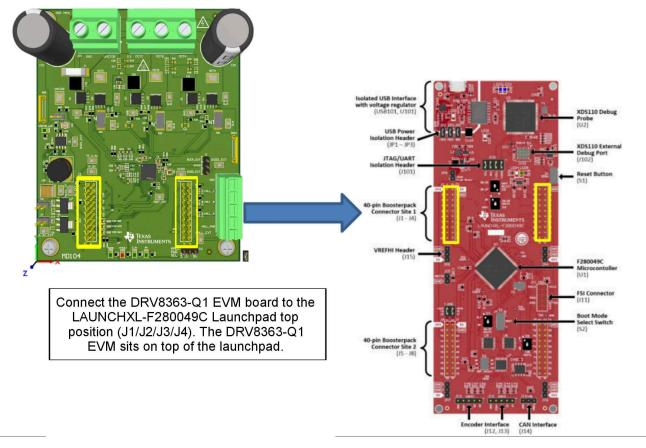
Figure 2-2. DRV8363-Q1EVM Mating to LAUNCHXL-F280049C
