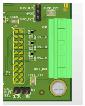
Figure 2-4. Hall Sensor Input and Power Connections (J11)
