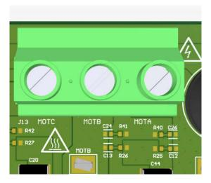
Figure 2-5. Motor Phase Connector (J13)
