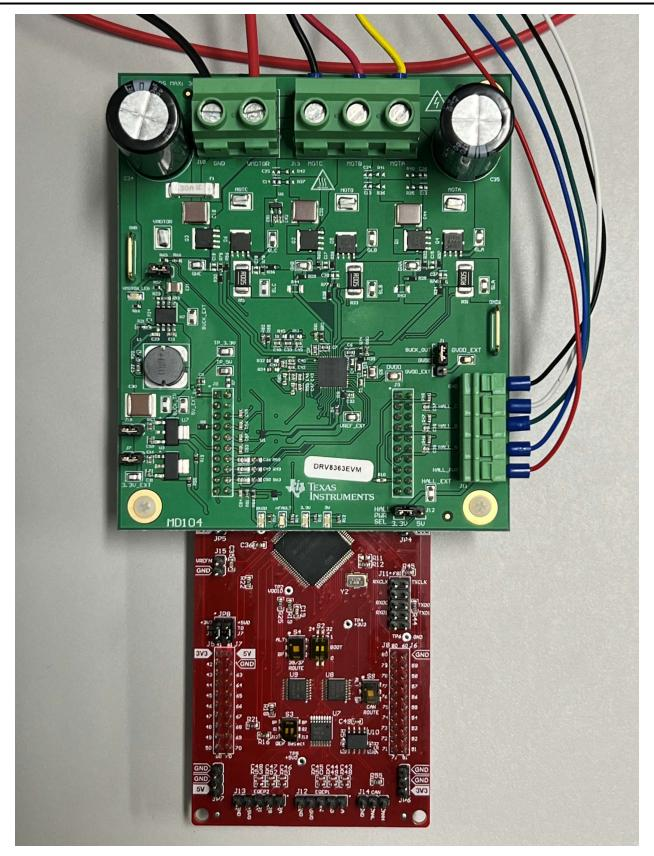
Figure 2-8. DRV8363-Q1EVM connected with Launch Pad
