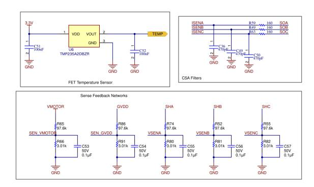
Figure 4-3. Schematic 3
