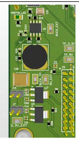
Figure 2-7. On-Board VMOTOR Buck, 3.3V LDO, and 5V LDO
