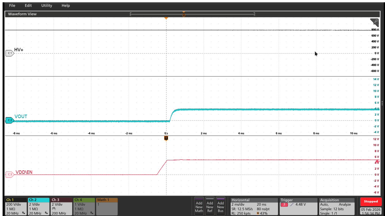
Figure 3-2. Voltage Sense Output (S2) Test Point at HV = 800V (EN = 5V)
