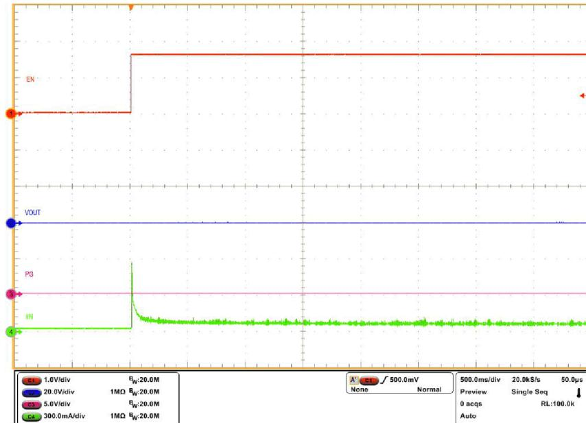
**Figure 3-4. Power Up Into Output Short Response of TPS1685EVM ( $V_{IN} = 54V$ , EN Stepped Up From 0V to 2V, and OUT Shorted to PGND)**
