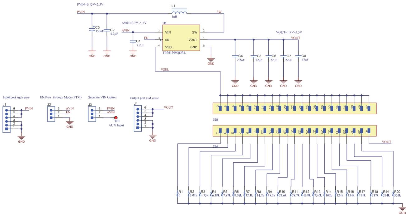
Figure 3-1. TPS61299EVM-016 Schematic
