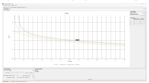
Figure 3-7. Adjusting I2T Trip Value
