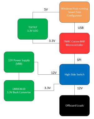
Figure 1-1. Block Diagram for HSS-HCMOTHERBRDEVM
