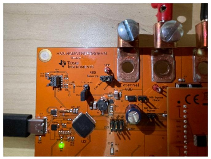
Figure 2-8. Configured for External VDD
