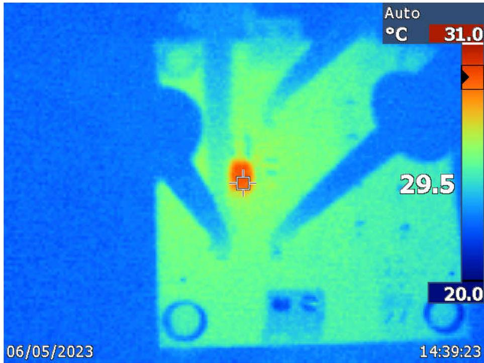
**Figure 5-2. IR Top Case Measurement**
