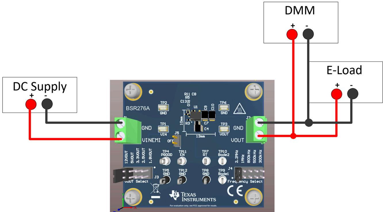
Figure 3-1. Test Setup Diagram
