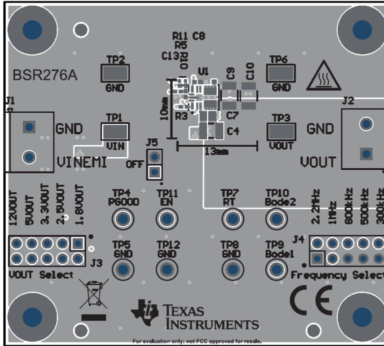
Figure 6-1. PCB Top 2-D (TPSM365R15EVM)
