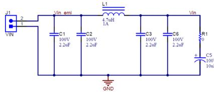
Figure 4-1. Schematic-Compliance Testing Filter
