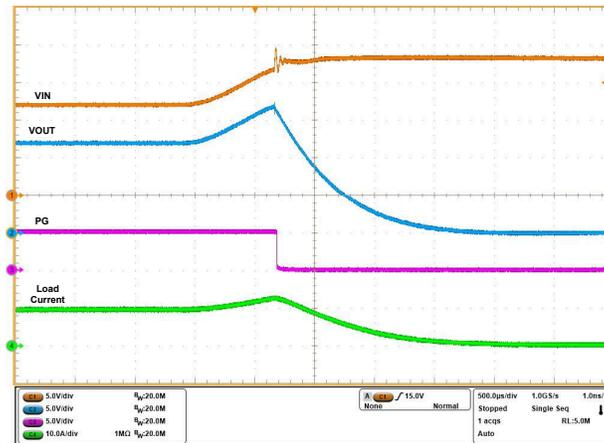
**Figure 5-8. Overvoltage Lockout Response of TPS25990 eFuse ( $V_{IN}$  Ramped Up from 12 V to 18 V,  $C_{OUT} = 470\ \mu\text{F}$ , and  $R_{LOAD} = 1.2\ \Omega$ )**
