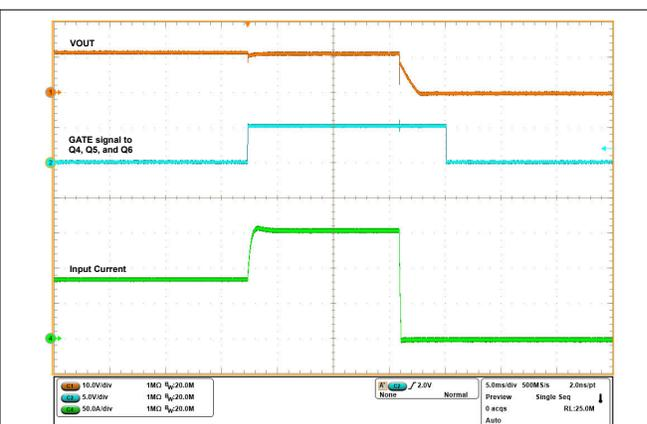
**Figure 5-14. Persistent Overload Performance in TPS25990EVM Using the Onboard Switching Circuit ( $V_{\text{IN}} = 12\ \text{V}$ ,  $t_{\text{TIMER}} = 14\ \text{ms}$ ,  $C_{\text{OUT}} = 1470\ \mu\text{F}$ ,  $R_{\text{IMON}} = 1.47\ \parallel\ 1.1\ \text{k}\Omega$ ,  $V_{\text{IREF}} = 1\ \text{V}$ ,  $I_{\text{OUT(Steady-State)}} = 85\ \text{A}$ , and  $I_{\text{OUT(Transient)}} = 65\ \text{A}$  for 18 ms)**
