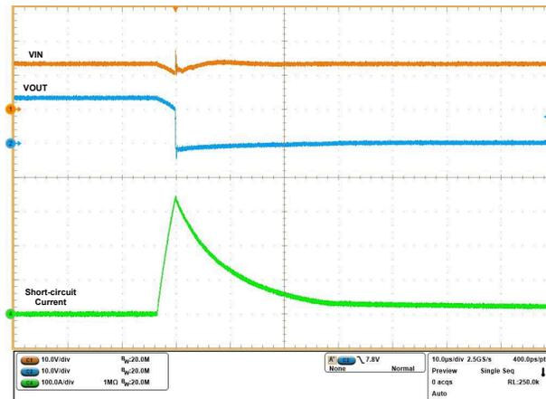
**Figure 5-15. Output Hot Short Response in TPS25990EVM ( $V_{IN} = 12\text{ V}$ ,  $R_{IMON} = 1.47\ \Omega \parallel 1.1\ \text{k}\Omega$ ,  $V_{REF} = 1\ \text{V}$ , and  $C_{OUT} = 10\ \mu\text{F}$ )**
