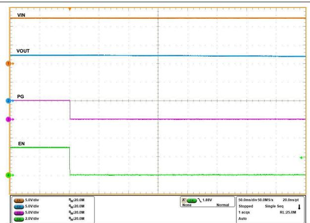
**Figure 5-17. QOD Disabled on TPS25990 eFuse ( $V_{IN} = 12\text{ V}$ ,  $C_{OUT} = 470\text{ }\mu\text{F}$ , and EN Pulled Low to 0 V)**
