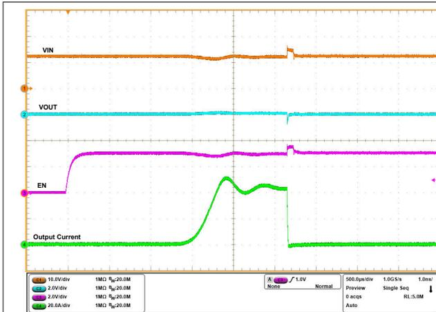
**Figure 5-6. Power Up into Output Short Response in TPS25990EVM ( $V_{IN} = 12\text{ V}$ , EN Stepped Up from 0 V to 3 V,  $R_{LIM}(TPS25990) = 665\ \Omega$ ,  $R_{LIM}(TPS25985) = 499\ \Omega$ ,  $V_{IREF} = 1\text{ V}$ , and OUT Shorted to PGND)**
