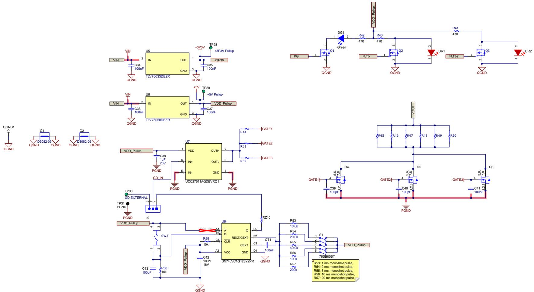
Figure 3-1. TPS25990EVM eFuse Evaluation Board Schematic
