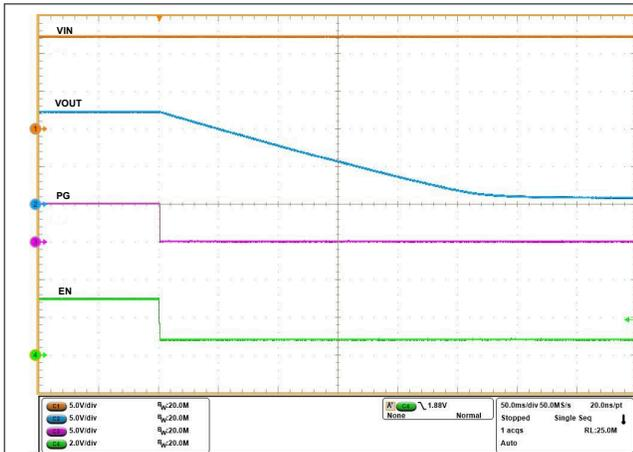
**Figure 5-16. QOD Enabled on TPS25990 eFuse ( $V_{IN} = 12\text{ V}$ ,  $C_{OUT} = 470\text{ }\mu\text{F}$ , and EN Pulled Low to 0.8 V)**
