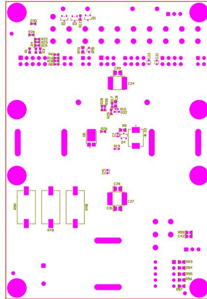
Figure 7-2. TPS25990EVM Board: Bottom Assembly
