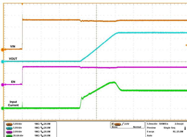
**Figure 5-2. Hot Plug Profile with TPS25990 eFuse and TPS25985 eFuse in Parallel ( $V_{IN}$  Stepped Up from 0 V to 12 V,  $C_{OUT} = 15.47 \text{ mF}$ ,  $C_{DVRT} = 33 \text{ nF}$ ,  $R_{LIM}(TPS25990) = 523 \Omega$ ,  $R_{LIM}(TPS25985) = 402 \Omega$ ,  $V_{REF} = 1 \text{ V}$ , and  $R_{LOAD} = 0.4 \Omega$ )**
