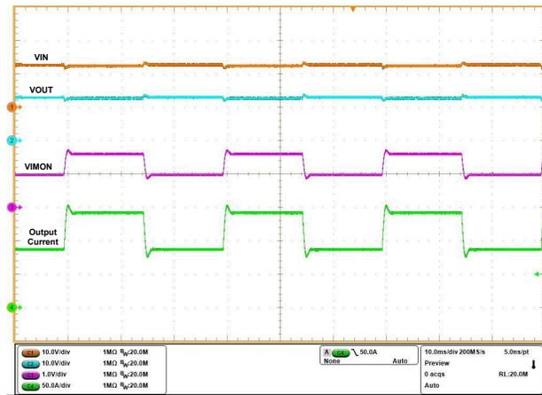
**Figure 5-9. Transient Overload Performance in TPS25990EVM ( $V_{IN} = 12\text{ V}$ ,  $t_{TIMER} = 20\text{ ms}$ ,  $C_{OUT} = 470\text{ }\mu\text{F}$ ,  $R_{IMON} = 1.47\text{ }\parallel\text{ }1.1\text{ k}\Omega$ ,  $V_{IREF} = 1\text{ V}$ ,  $I_{OUT}$  Ramped from 85 A to 140 A then 85 A within 15 ms)**
