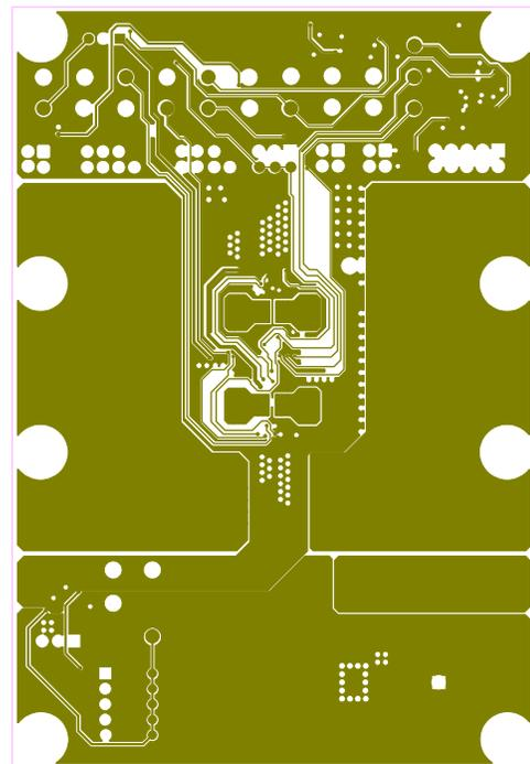
Figure 7-8. TPS25990EVM Board: Layer 5 (Signal)
