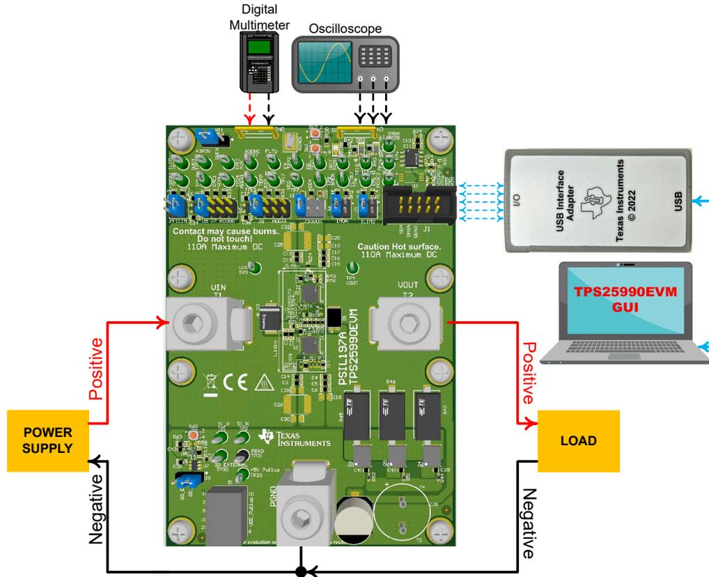
**Figure 5-1. TPS25990EVM Setup with Test Equipment**
