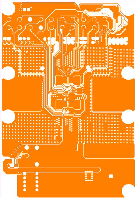
Figure 7-7. TPS25990EVM Board: Layer 4 (Signal)
