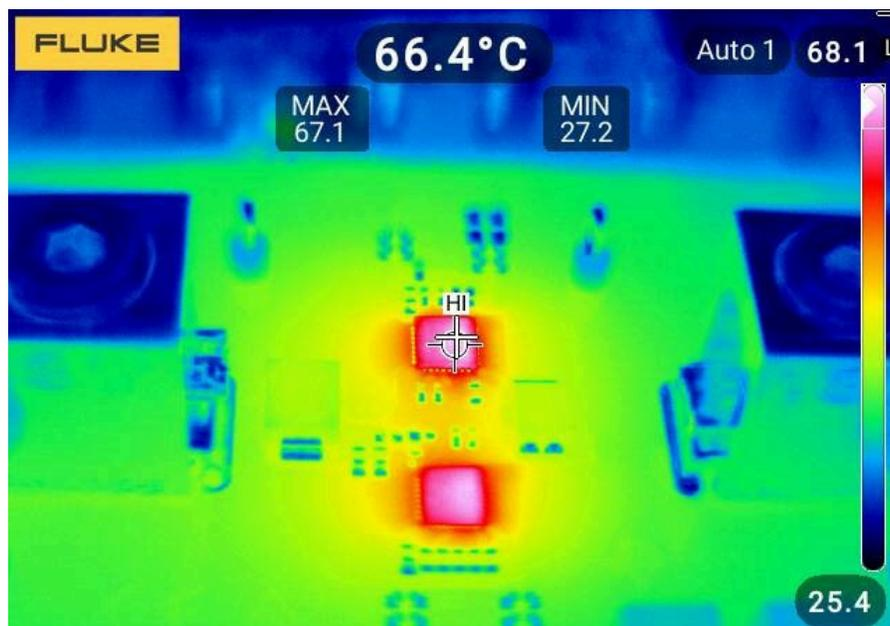
Figure 5-18. Thermal Performance in TPS25990EVM ( $V_{IN} = 12$  V,  $R_{IMON} = 0.91 \parallel 1.1$  k $\Omega$ ,  $V_{IREF} = 1.13$  V, and  $I_{OUT} = 110$  A)
