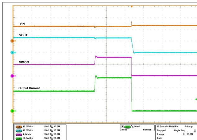
**Figure 5-11. Overcurrent Performance in TPS25990EVM ( $V_{IN} = 12\text{ V}$ ,  $t_{TIMER} = 20\text{ ms}$ ,  $C_{OUT} = 470\text{ }\mu\text{F}$ ,  $R_{IMON} = 1.47\text{ }\parallel\text{ }1.1\text{ k}\Omega$ ,  $V_{IREF} = 1\text{ V}$ ,  $I_{OUT}$  Ramped from 85 A to 140 A then 85 A within 30 ms)**
