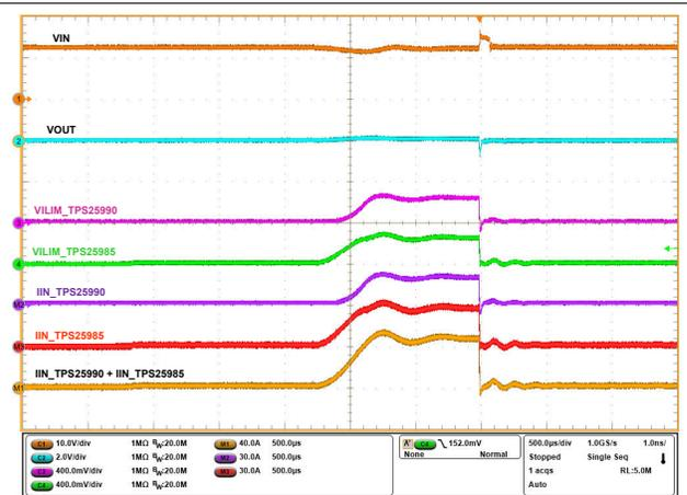
**Figure 5-7. Power Up into Output Short Response in TPS25990EVM: Current Sharing between TPS25990 and TPS25985 eFuses ( $V_{IN} = 12\text{ V}$ , EN Stepped Up from 0 V to 3 V,  $R_{LIM}(TPS25990) = 665\ \Omega$ ,  $R_{LIM}(TPS25985) = 499\ \Omega$ ,  $V_{IREF} = 1\text{ V}$ , and OUT Shorted to PGND)**
