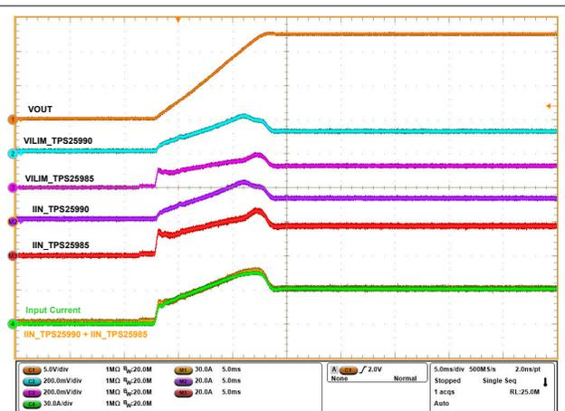
**Figure 5-4. Start-up Profile with ENABLE: Current Sharing between TPS25990 and TPS25985 eFuses ( $V_{IN} = 12$  V, EN Stepped Up from 0 V to 3 V,  $C_{OUT} = 15.47$  mF,  $R_{LOAD} = 0.4$   $\Omega$ ,  $R_{ILIM}(TPS25990) = 523$   $\Omega$ ,  $R_{ILIM}(TPS25985) = 402$   $\Omega$ ,  $V_{IREF} = 1$  V, and  $C_{DVDT} = 33$  nF)**
