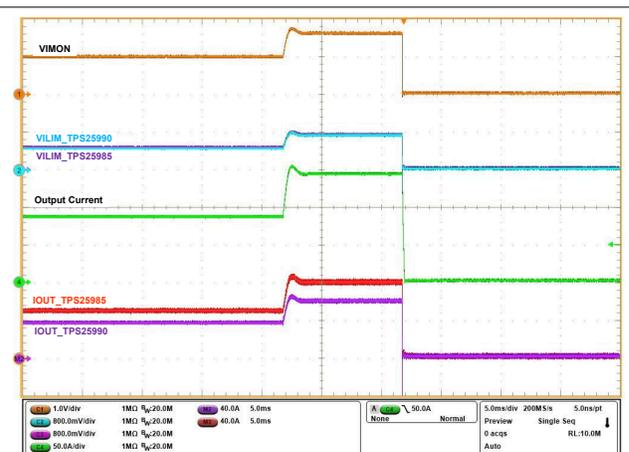
**Figure 5-12. Overcurrent Performance in TPS25990EVM: Current Sharing between TPS25990 and TPS25985 eFuses ( $V_{IN} = 12\text{ V}$ ,  $t_{TIMER} = 10\text{ ms}$ ,  $C_{OUT} = 470\text{ }\mu\text{F}$ ,  $R_{IMON} = 1.47\text{ }\parallel\text{ }1.1\text{ k}\Omega$ ,  $V_{IREF} = 1\text{ V}$ ,  $I_{OUT}$  Ramped from 85 A to 140 A then 85 A within 15 ms)**
