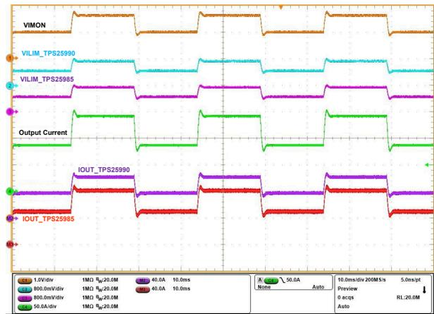
**Figure 5-10. Transient Overload Performance in TPS25990EVM: Current Sharing between TPS25990 and TPS25985 eFuses ( $V_{IN} = 12\text{ V}$ ,  $t_{TIMER} = 20\text{ ms}$ ,  $C_{OUT} = 470\text{ }\mu\text{F}$ ,  $R_{IMON} = 1.47\text{ }\parallel\text{ }1.1\text{ k}\Omega$ ,  $V_{IREF} = 1\text{ V}$ ,  $I_{OUT}$  Ramped from 85 A to 140 A then 85 A within 15 ms)**
