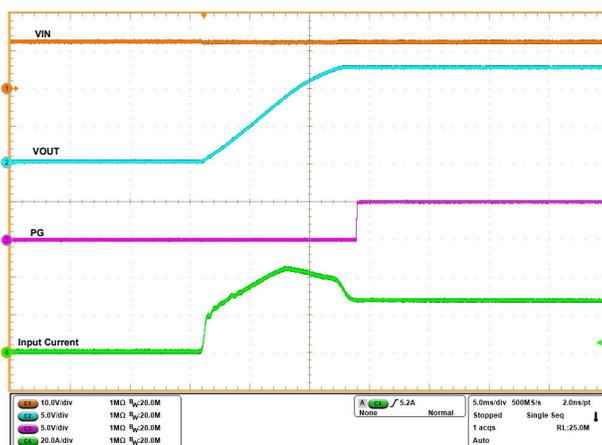
Figure 5-5. Start-up with Current Limit Response in TPS25990EVM ( $V_{IN} = 12 \text{ V}$ , EN Stepped Up from 0 V to 3 V,  $R_{LIM}(TPS25990) = 665 \Omega$ ,  $R_{LIM}(TPS25985) = 499 \Omega$ ,  $V_{IREF} = 1 \text{ V}$ ,  $C_{OUT} = 18.47 \text{ mF}$ ,  $R_{LOAD} = 0.45 \Omega$ , and  $C_{DVRT} = 33 \text{ nF}$ )
