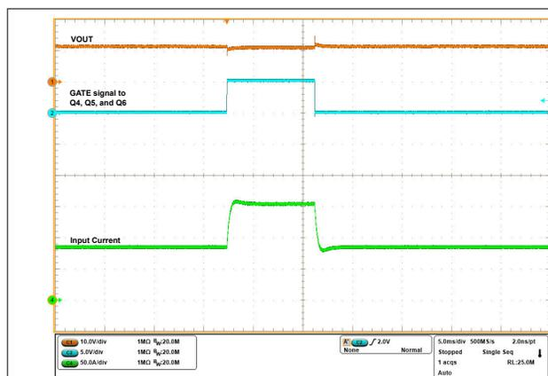
**Figure 5-13. Transient Overload Performance in TPS25990EVM Using the Onboard Switching Circuit ( $V_{\text{IN}} = 12\ \text{V}$ ,  $t_{\text{TIMER}} = 14\ \text{ms}$ ,  $C_{\text{OUT}} = 1470\ \mu\text{F}$ ,  $R_{\text{IMON}} = 1.47\ \parallel\ 1.1\ \text{k}\Omega$ ,  $V_{\text{IREF}} = 1\ \text{V}$ ,  $I_{\text{OUT(Steady-State)}} = 85\ \text{A}$ , and  $I_{\text{OUT(Transient)}} = 65\ \text{A}$  for 9 ms)**
