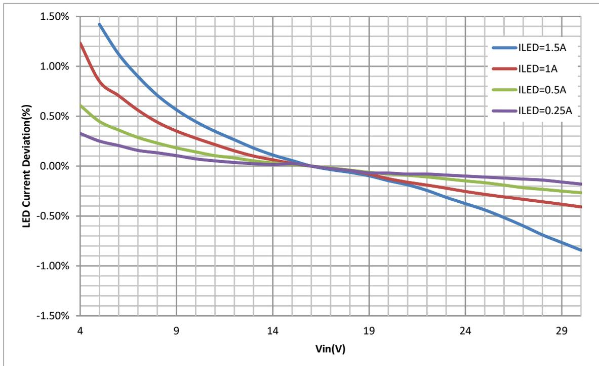
Figure 4-4. LED Current Deviation vs. Input Voltage in Analog Dimming Mode, 1 WLED
