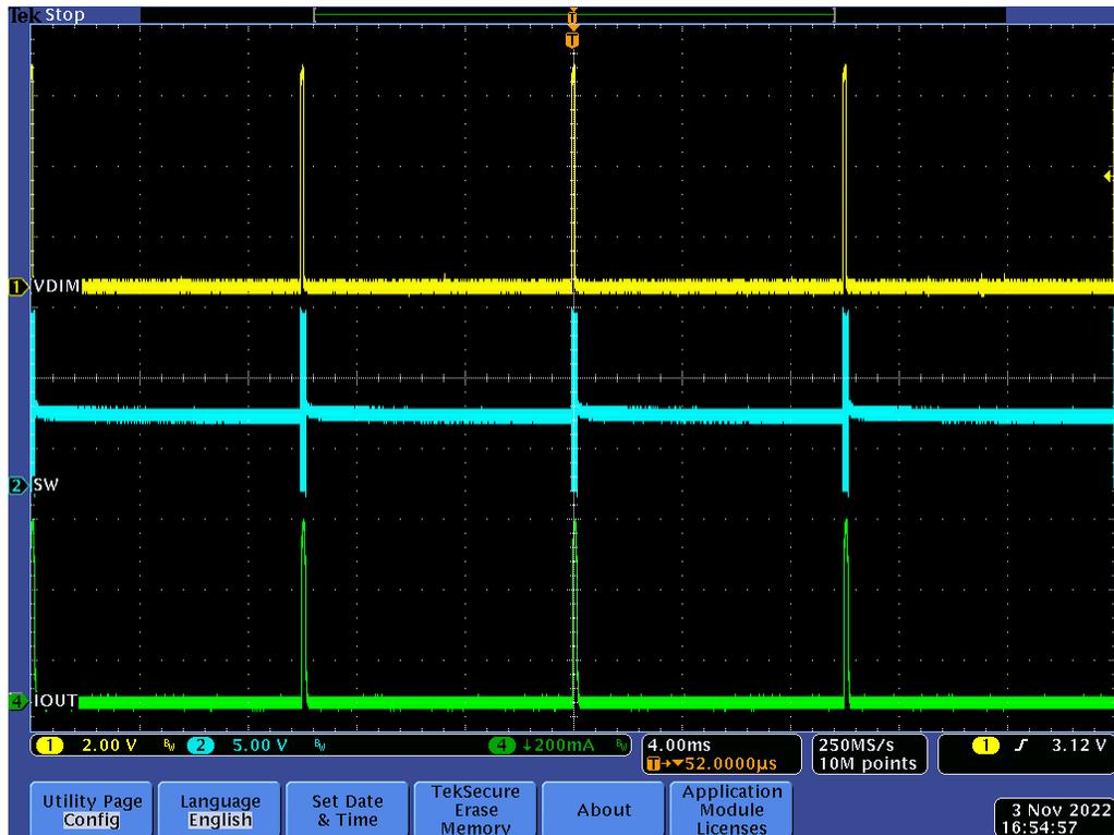
Figure 4-8. 1% Duty Cycle 100-Hz PWM Dimming(TPS92200D1RXLR)
