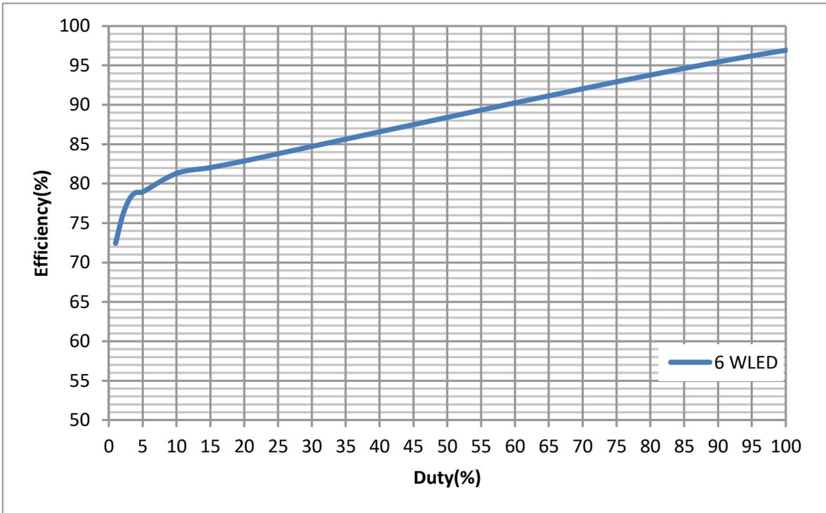
**Figure 4-2. Efficiency vs. PWM Duty Cycle in PWM Dimming Mode(TPS92200D1RXLR), 1.0 A at 100% Duty**
