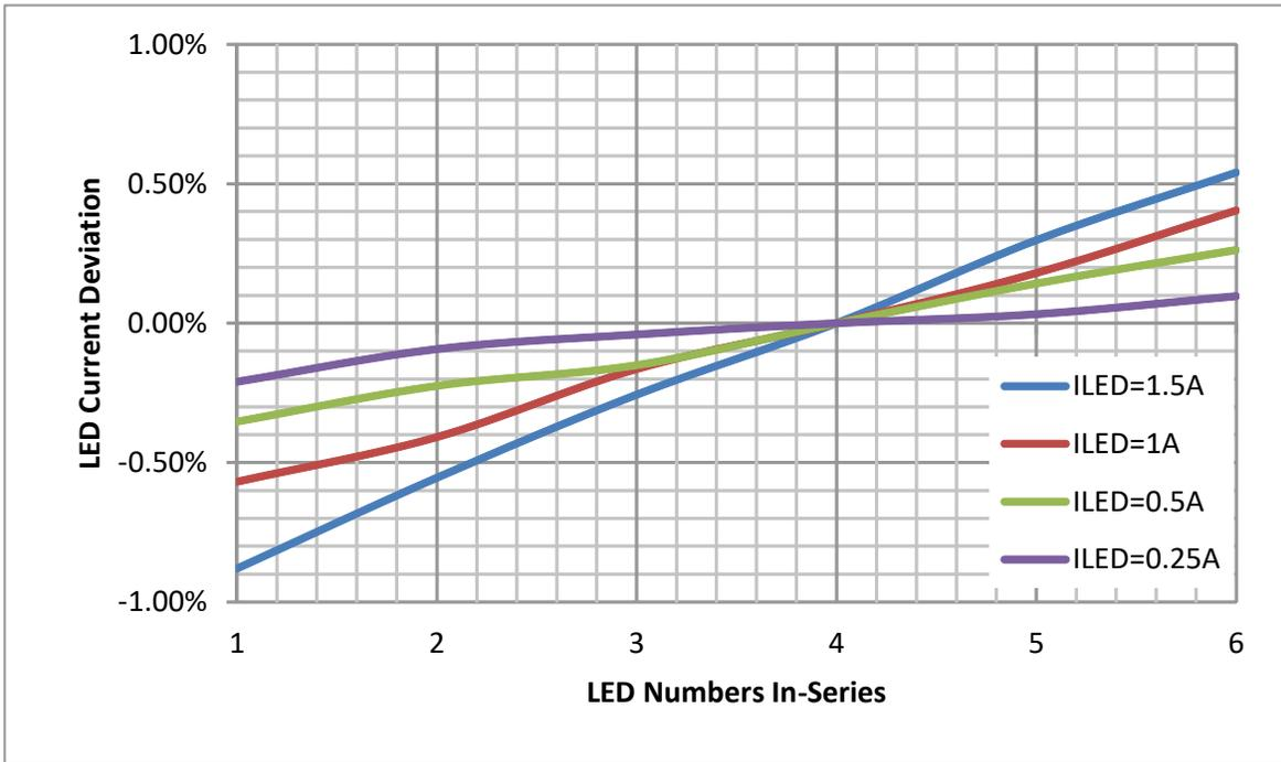
Figure 4-5. LED Current Deviation vs. LED Numbers in Series in Analog Dimming Mode,  $V_{IN} = 24\text{ V}$
