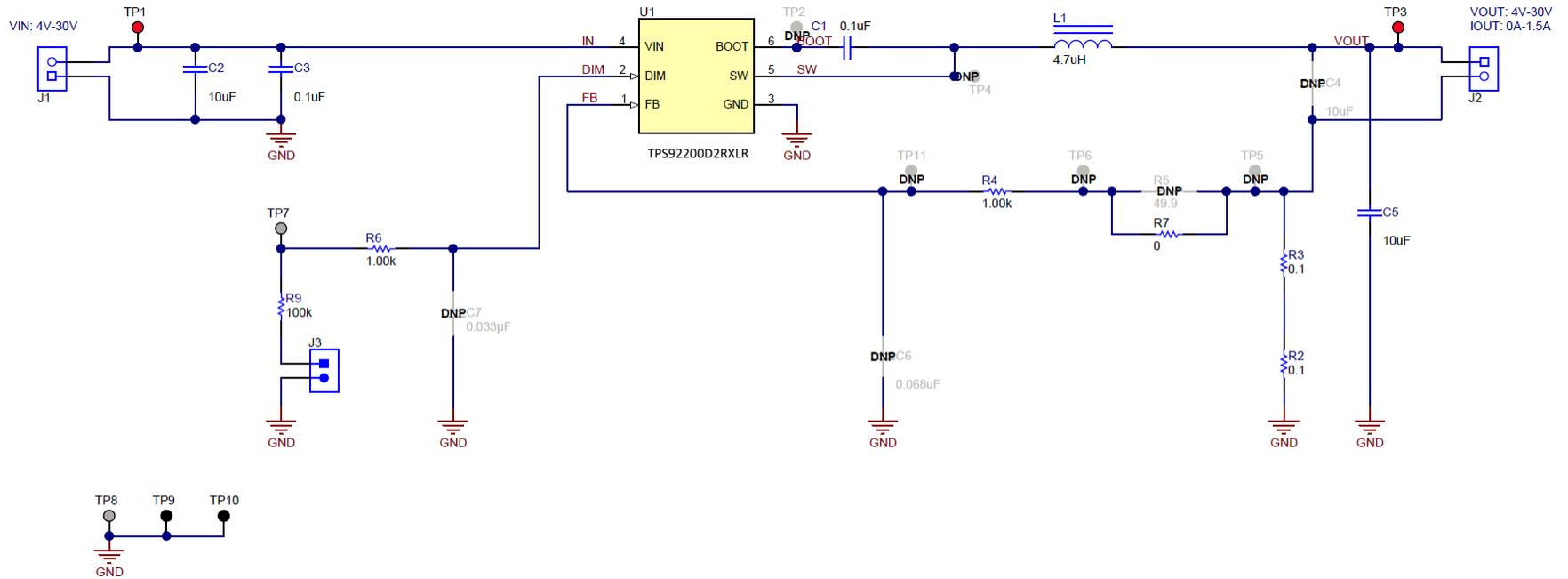
Figure 5-2. TPS92200D2RXLREVM Schematic
