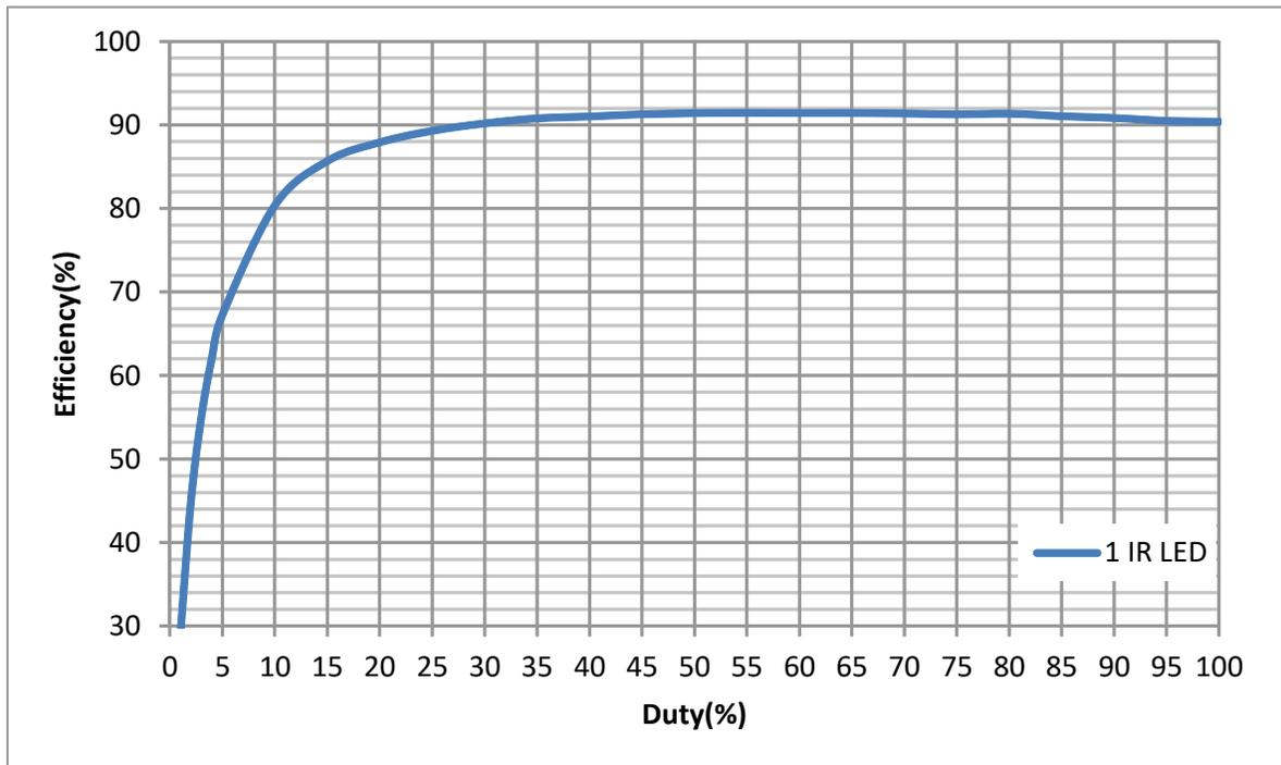
**Figure 4-3. Efficiency vs. PWM Duty Cycle in Analog Dimming Mode(TPS92200D2RXLR)**
