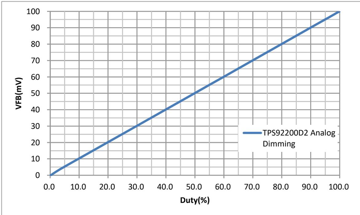
Figure 4-7. Output Current ratio vs PWM Duty Cycle in Analog Dimming Mode(TPS92200D2RXLR)
