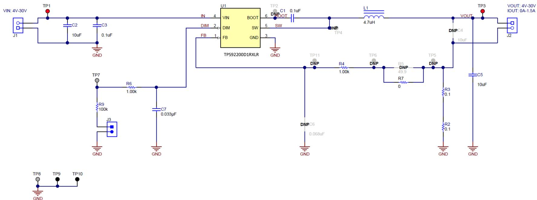
Figure 5-1. TPS92200D1RXLREVM Schematic
