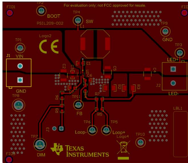
Figure 6-1. Top Layer and Top Overlay (Top View)
