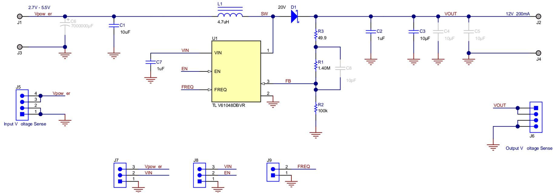
Figure 1. TLV61048EVM-042 Schematic
