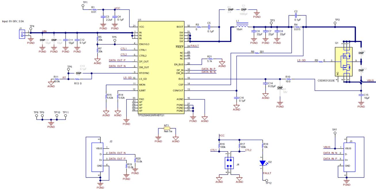
Figure 8. TPS25840Q1EVM-079 Schematic
