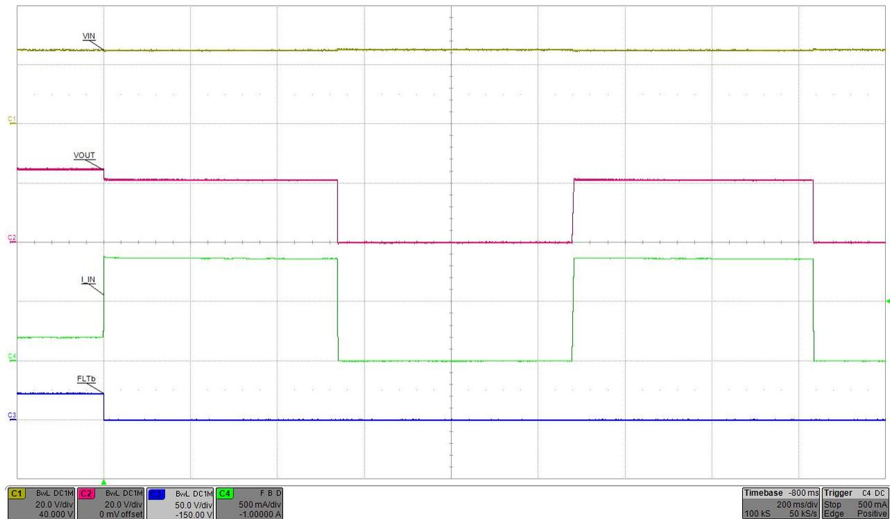
Figure 3. J4 = 1-2 Position, Current Limit (800 mA) and Auto-Retry
