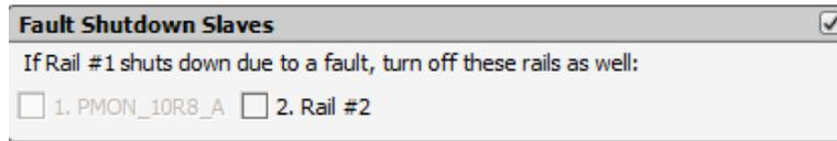
Figure 4-31. Fault Shutdown Slaves
