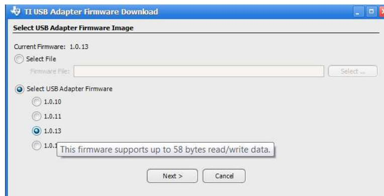
**Figure 2-5. Adapter Firmware Download Tool (2/2)**
