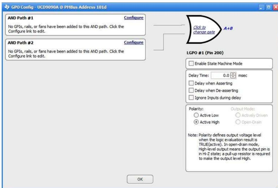
Figure 4-15. Add Logic-Controlled GPO
