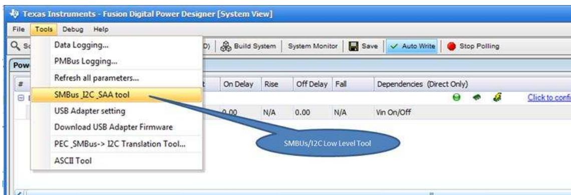
Figure 6-13. SMBUS, I2C, and SAA Toolbar Launch
