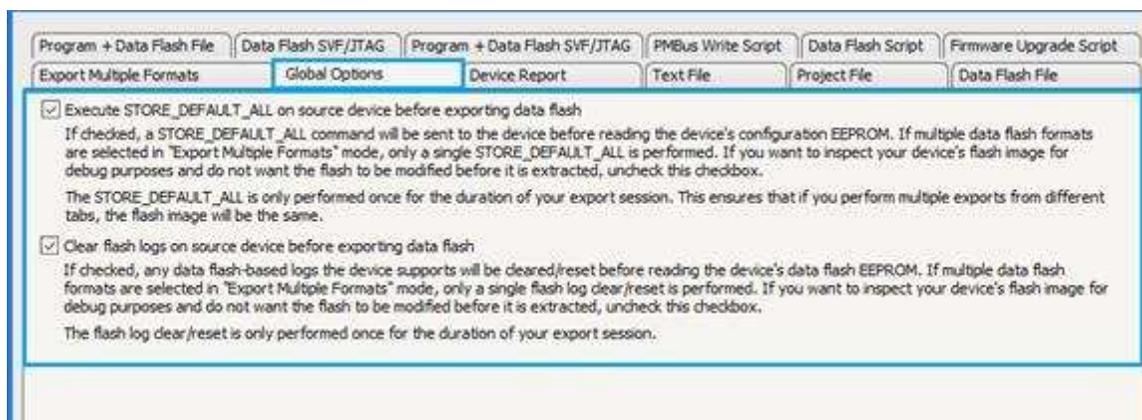
**Figure 5-1. Configuration Storage Setting**
