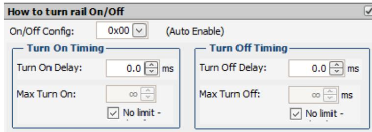
**Figure 4-28. Rail On/Off Config Setting (1/2)**
