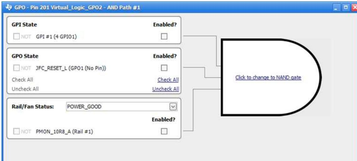
Figure 4-16. Logic GPO Input Selection
