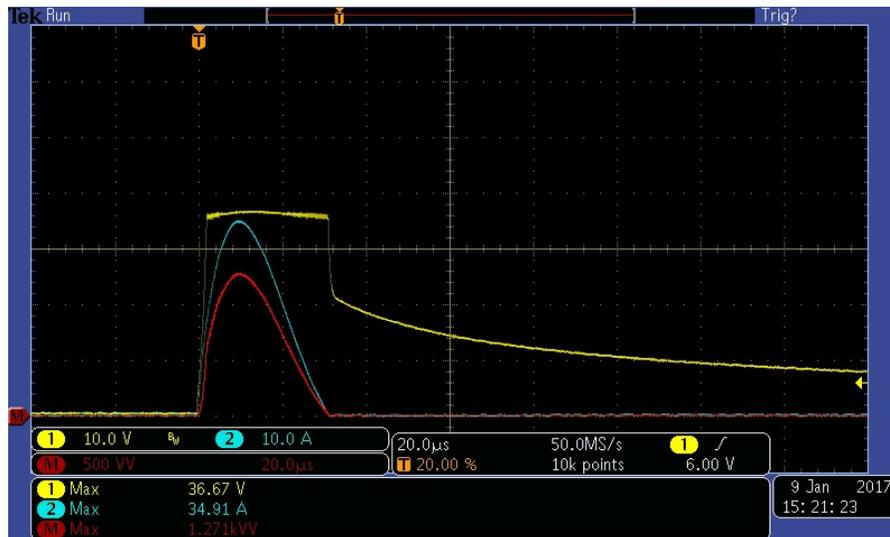
Figure 6. TVS3300DRV Surge Test Waveform
