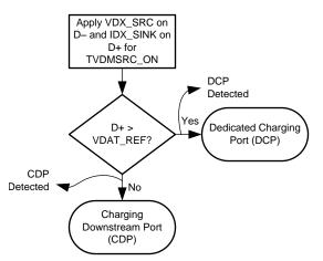
Figure 12-4. Secondary Detection
