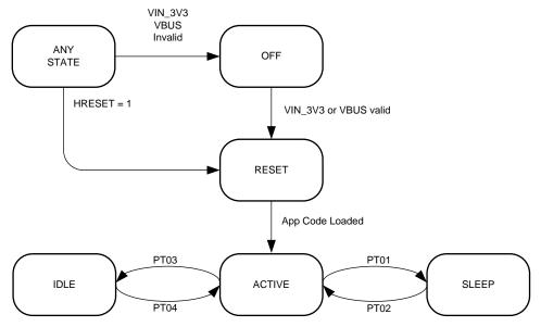
Figure 5-1. Power State Diagram
