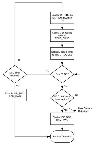
Figure 12-2. Data-Contact Detect (DCD)
