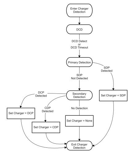
Figure 12-1. Charger-Detection State Machine
