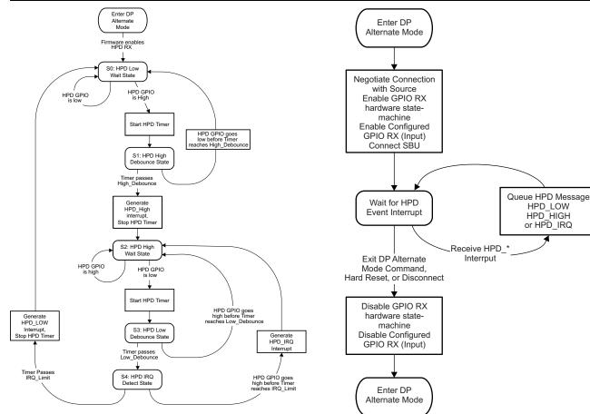
Figure 10-1. DisplayPort Sink-Side Hardware Flow (HPD RX)
