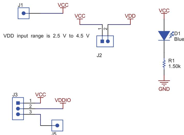
VDDIO can be separate supply for GPIO pins
