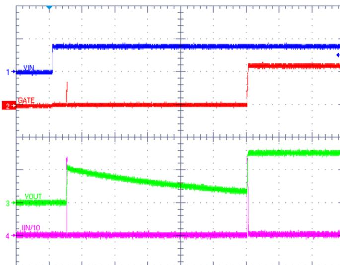
**Figure 17. Inrush Current with 4900- $\mu$ F Output Capacitor**
