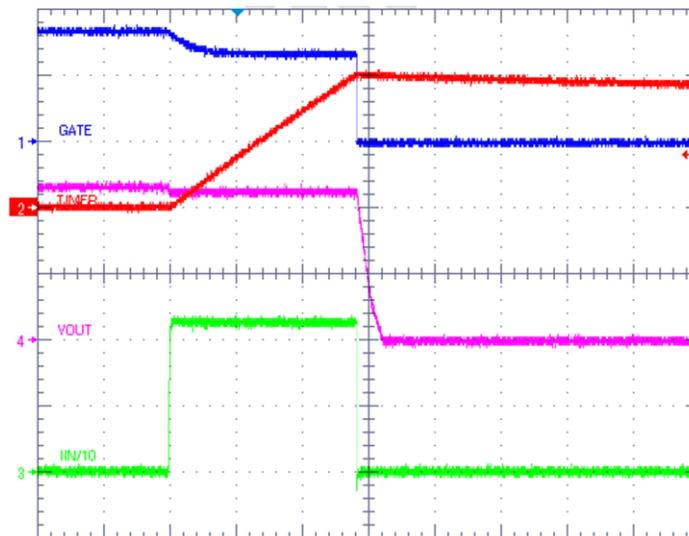
**Figure 8. Fault Timeout**
