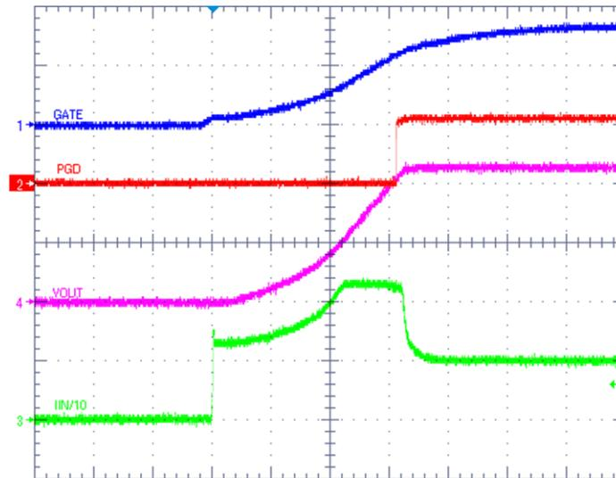
**Figure 11. Turn-on Sequence with 1-A Load Current**
