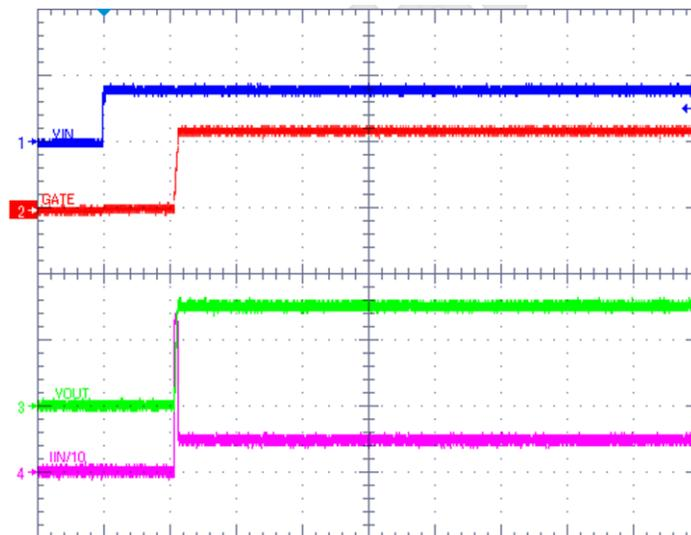
Figure 16. Inrush Current with 2550- $\mu$ F Output Capacitor
