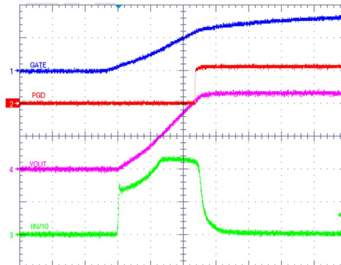
**Figure 10. Turn-on Sequence with No Load Current**
