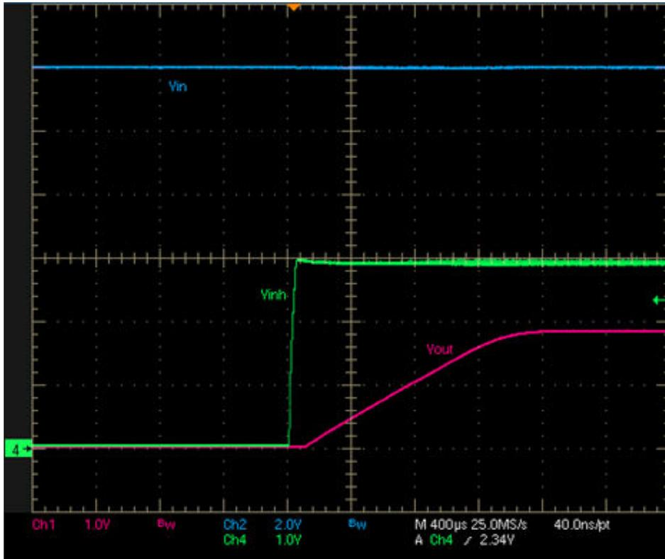
Figure 6-3. INH Start-Up Waveform
