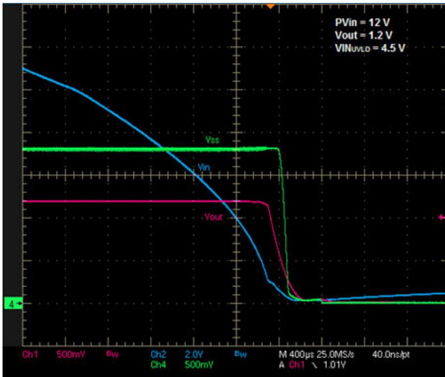
Figure 6-2. UVLO Shutdown Waveform
