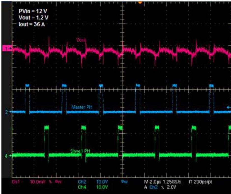
Figure 6-6. Output Voltage Ripple – 180° Out-of-Phase
