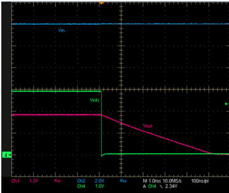
Figure 6-4. INH Shutdown Waveform
