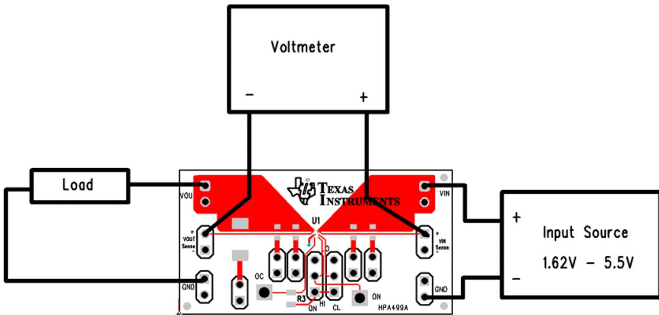
Figure 1.  $r_{ON}$  Setup
