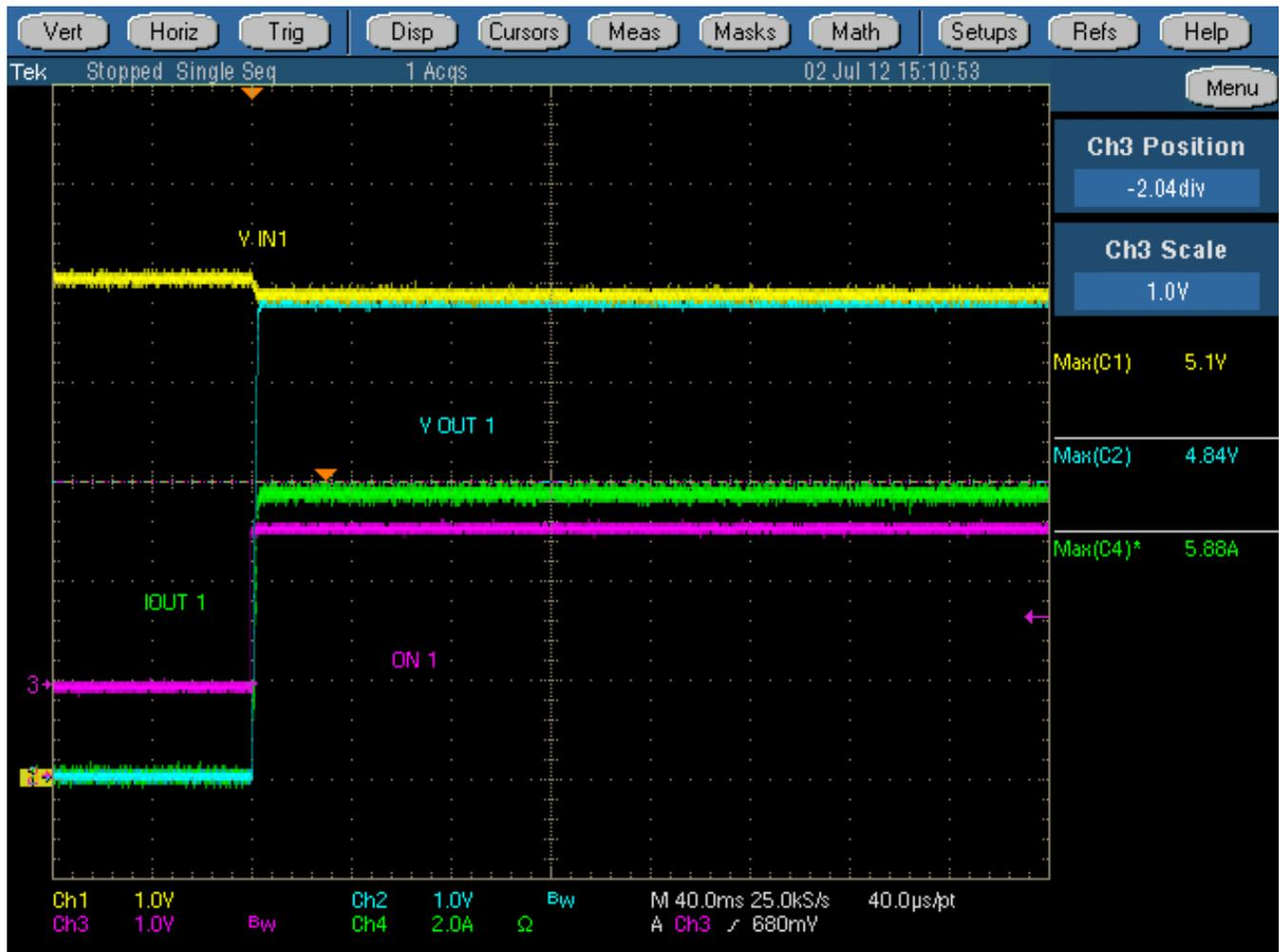
Figure 8. TPS22965EVm-023 Turn-ON and Operation at 6 A
