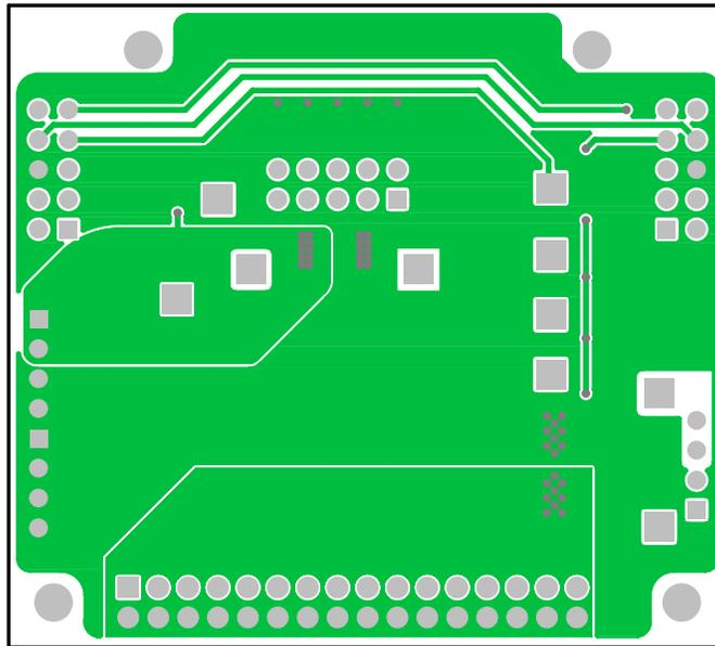
Figure 5. TLC59282 EVM Bottom Copper (Viewed From Bottom)
