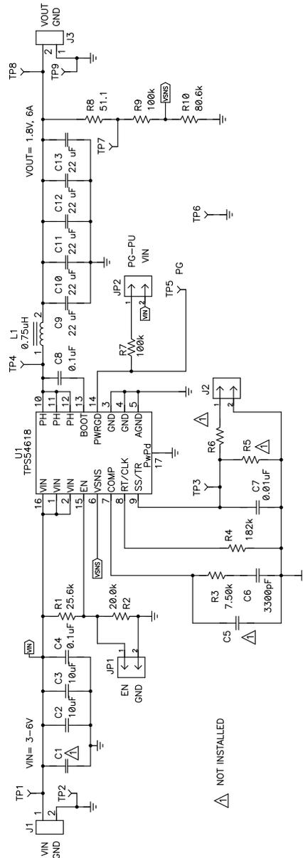
Figure 16. TPS54618EVM-606 Schematic
