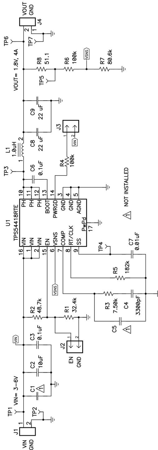
Figure 16. TPS54418EVM-375 Schematic
