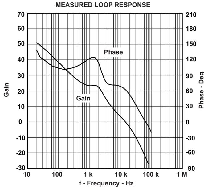
Figure 5. Measured Loop Response, TPS5450, VIN = 25 V
