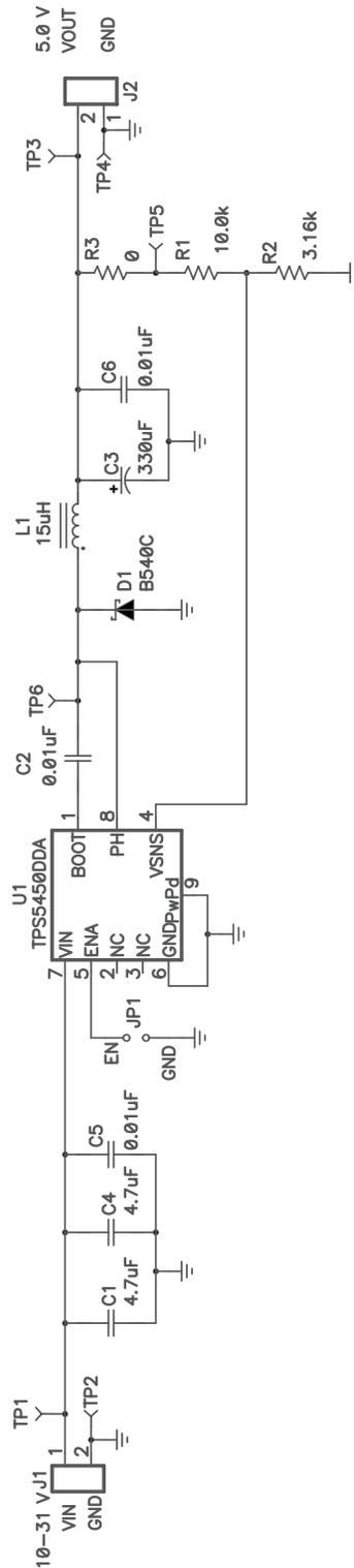
**Figure 13. TPS5450EVM-254 Schematic**
