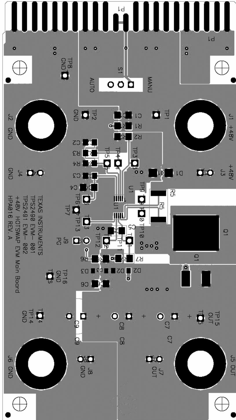
Test points are provided throughout the EVM main board for monitoring. The test points are listed in Table 4–2.
