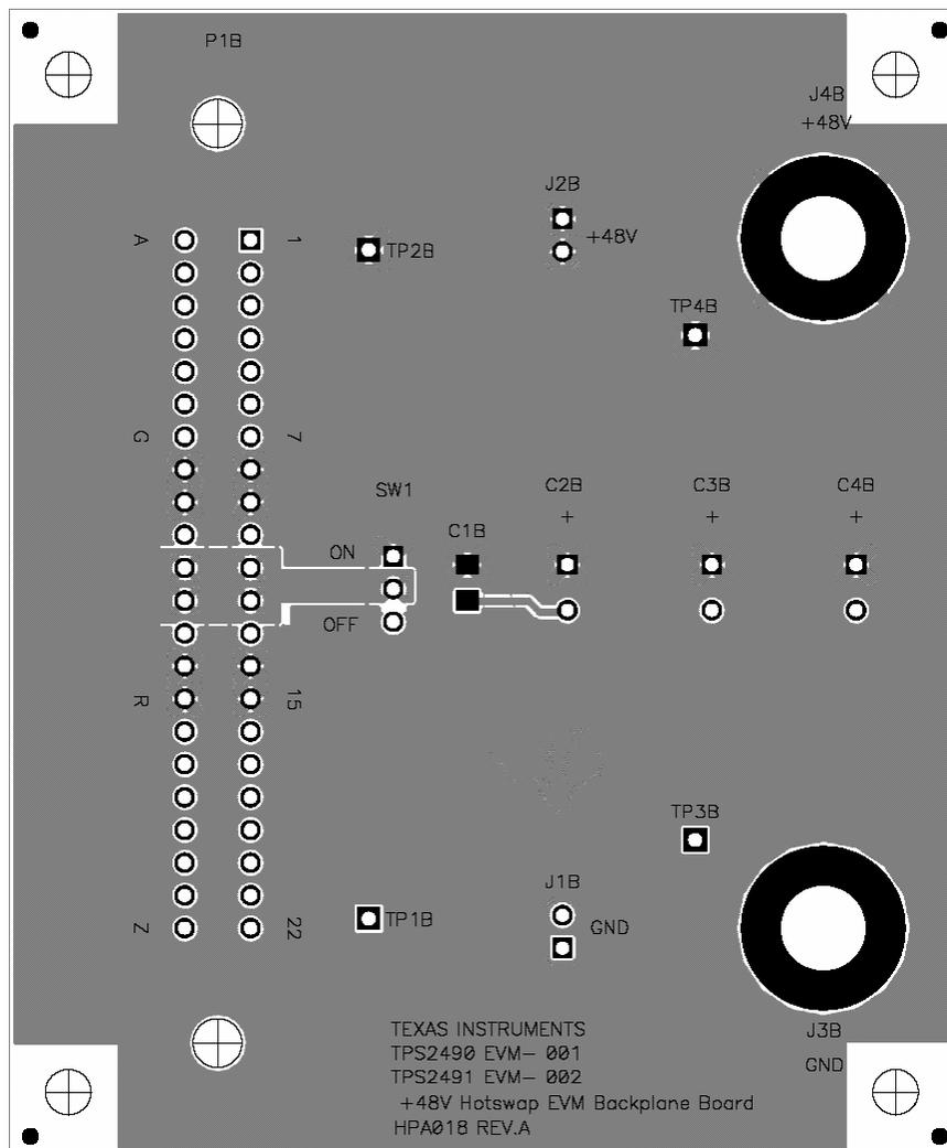
Test points are also provided throughout the EVM backplane board for monitoring as listed in Table 4–1.
