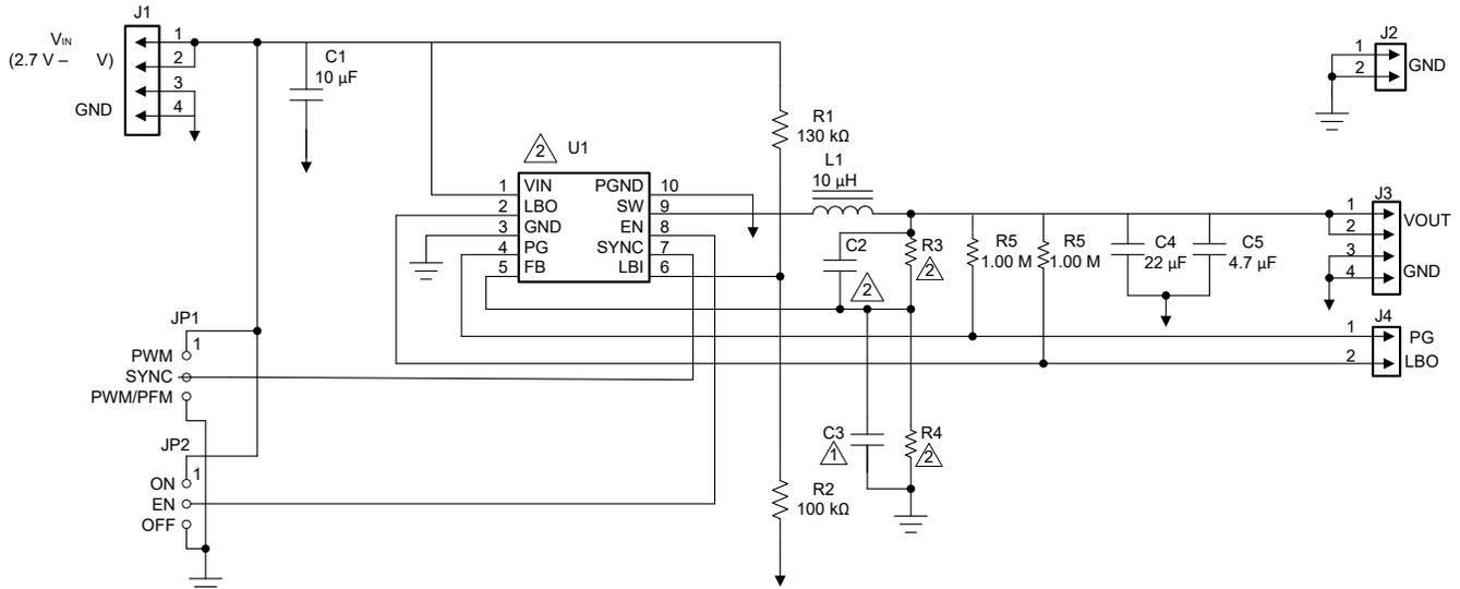
Figure 3-1. TPS6205xEVM Schematic
