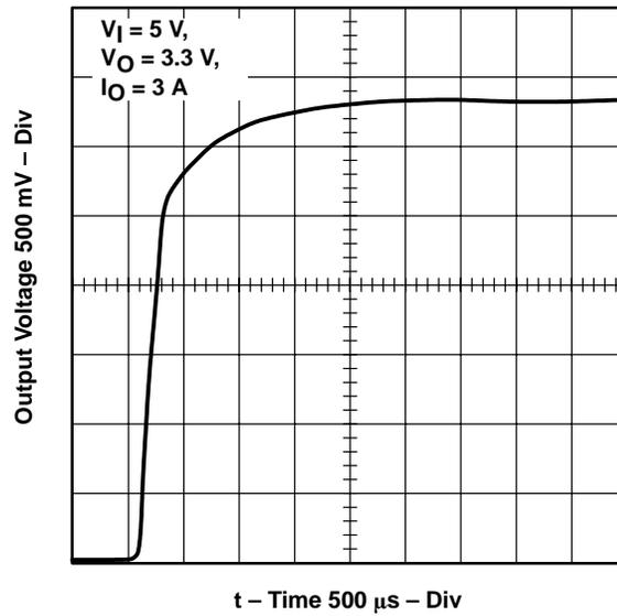
Figure 1–10. SLVP101 (3.3 V Output) Startup (No Load)
