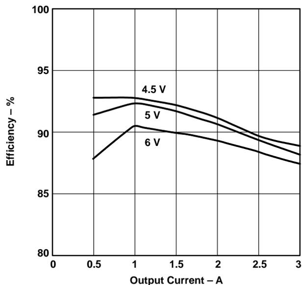
Figure 1–8. Measured SLVP103 (1.8 V Output) Efficiency vs. Load
