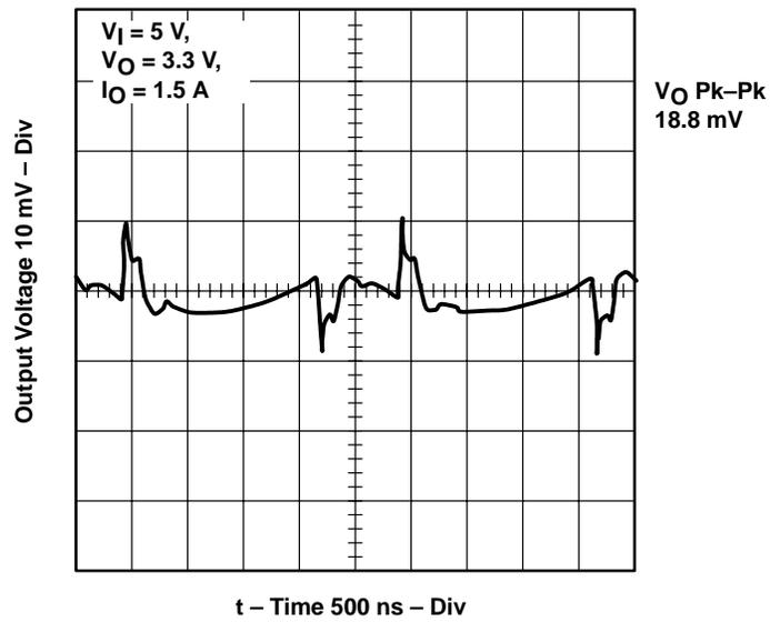
Figure 1–13. SLVP101 (3.3 V Output) Pulse Load Response
