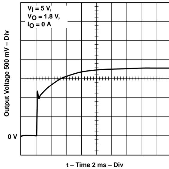
Figure 1–17. SLVP103 Startup (1.8 V Output) (Resistive Load)
