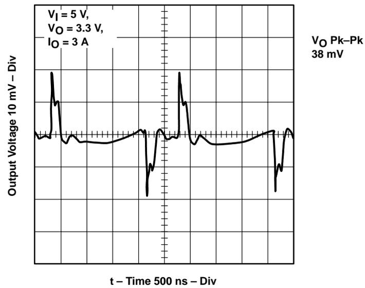
Figure 1–12. SLVP101 (3.3 V Output) 50% Load Output Voltage Ripple
