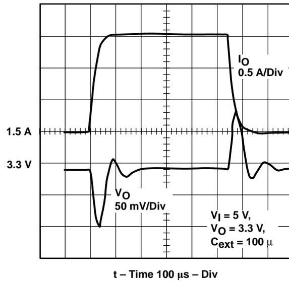
Figure 1–14. SLVP101 (3.3 V Output) CR1 Cathode Switching Waveform
