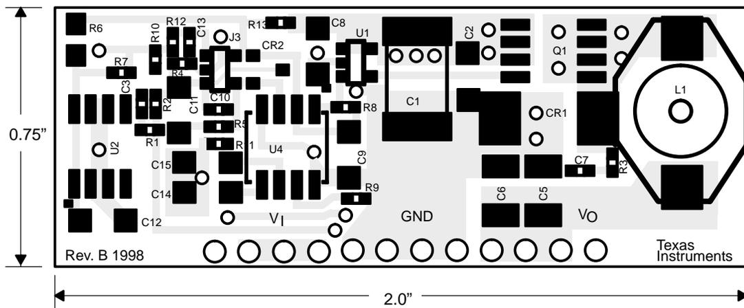
Figure 1–5. Component-Side Copper
