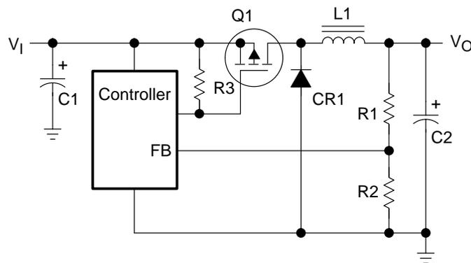
The SLVP101, SLVP102, and SLVP103 buck converters use the Texas Instruments TL5001 PWM controller to give power supply outputs of 3.3 V, 2.5 V, and 1.8 V at 0 to 3 A. Also featured in this design are the TL1431 reference IC, the TPS2817 MOSFET driver IC, and the TLV2231 operational amplifier. These converters operate over an input voltage range of 4.5 V to 9 V with typical efficiencies of 90 percent for 3.3 V out and 80 percent for 1.8 V out.
