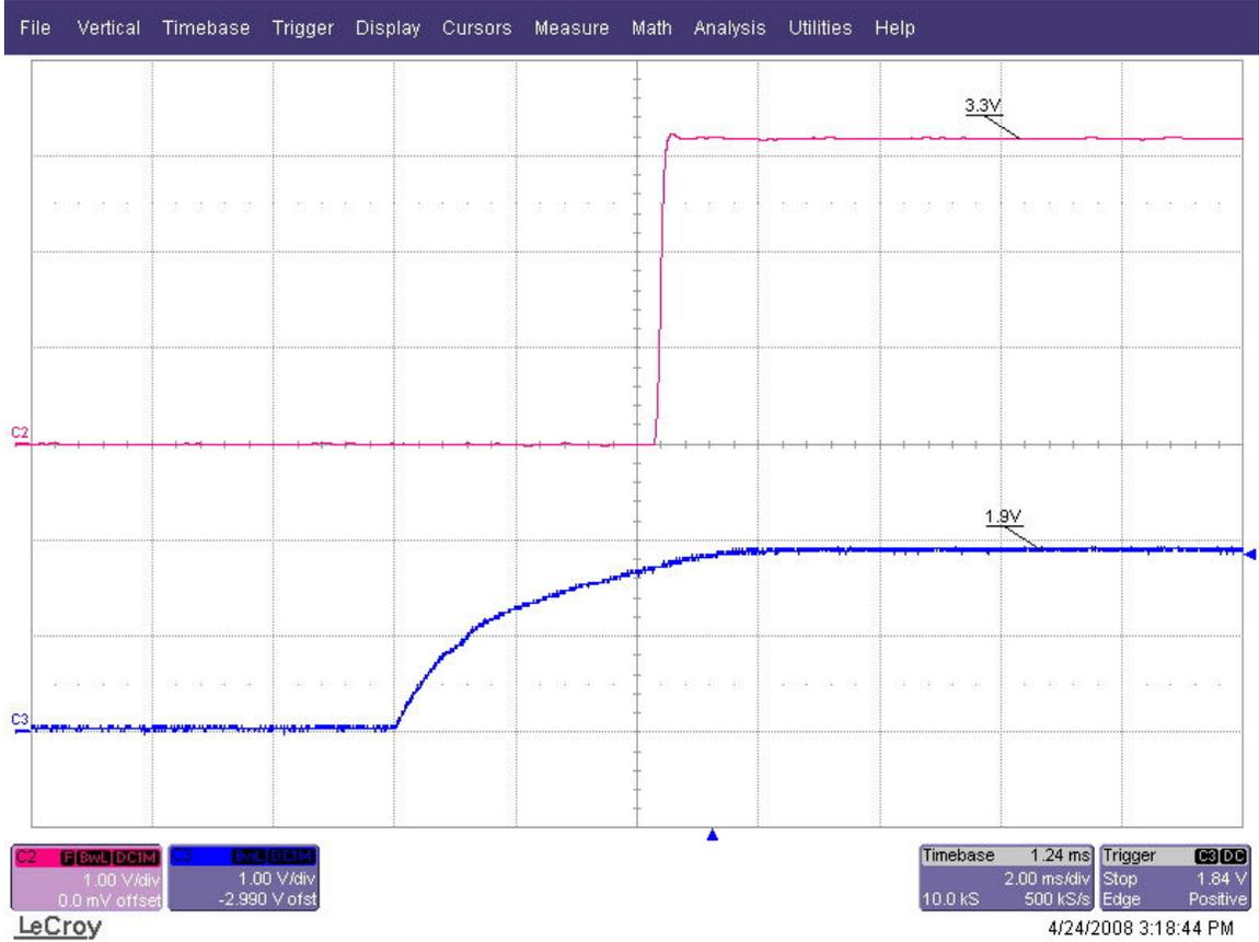
Figure 1. Power Up with 12-V Input
