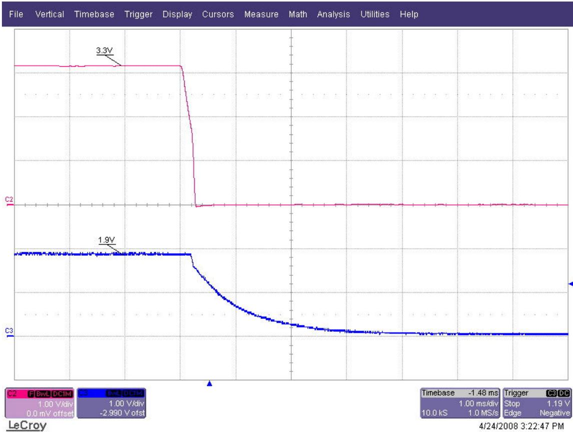
Figure 3. Power Down with 12-V Input
