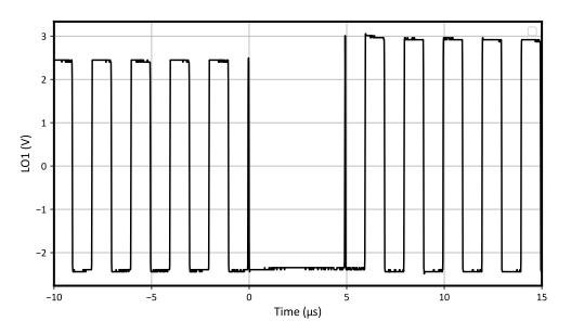
Figure 8-2. LO SET Run 37 (IIM-Disabled Mode, f<sub>sw</sub> = 500kHz)
