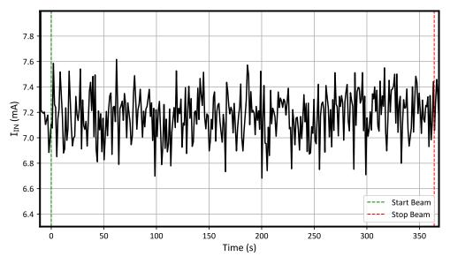
Figure 7-10. SEB On Run 25 (IIM-Disabled Mode, PWM/LI = 14V)
