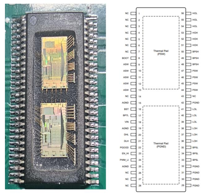
Figure 3-1. Photograph of Delidded TPS7H6005-SP (Left) and Pinout Diagram (Right)
