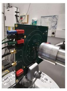
Figure 4-1. Photograph of the TPS7H60x5-SP Evaluation Board in Front of the Heavy-lon Beam Exit Port at the Texas A&M Cyclotron
