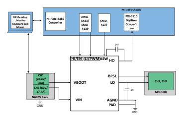
Figure 6-1. Block Diagram of the SEE Test Setup for the TPS7H60x5-SP
