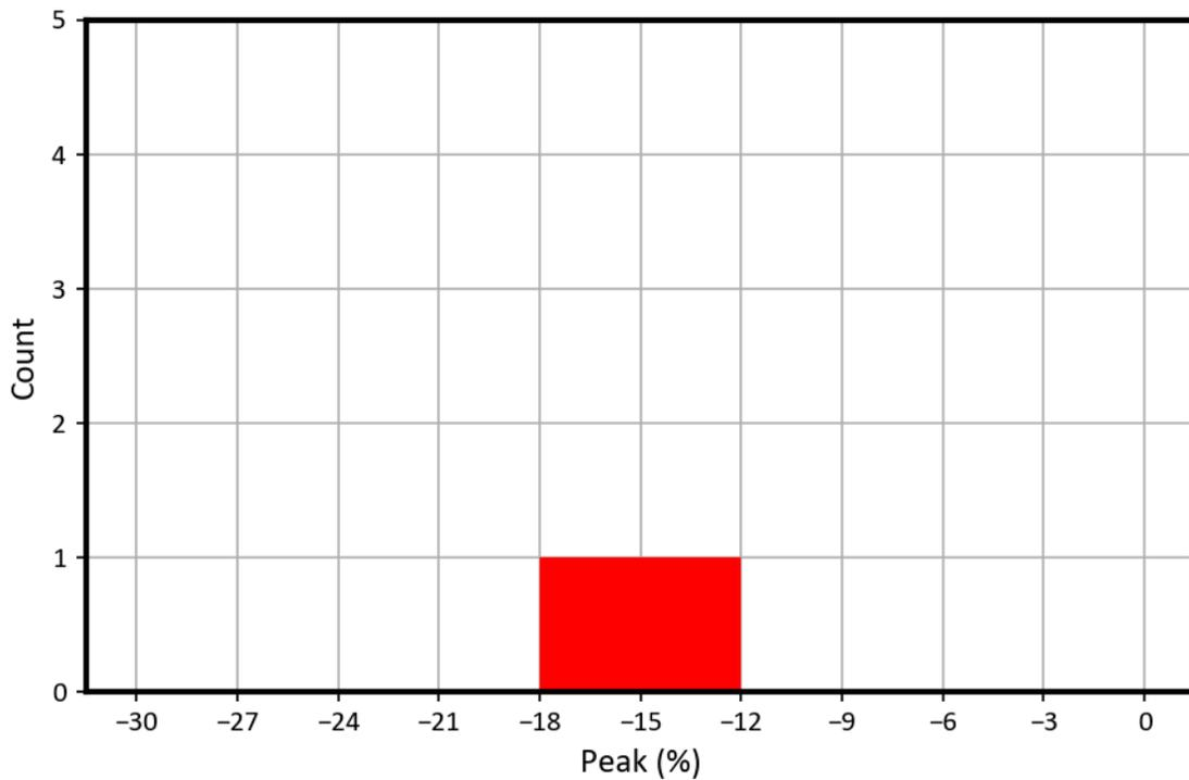
Figure 7-5. Histogram of the Normalized Amplitude for the Positive and Negative  $V_{OUT}$  SETs on Run # 6
