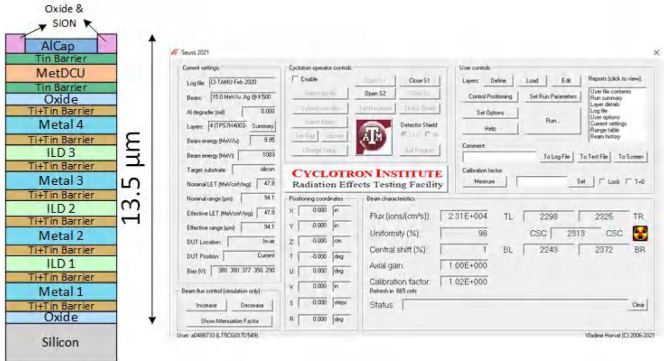
**Figure 5-1. Generalized Cross-Section of the LBC8 Technology BEOL Stack on the TPS7H4003-SEP [Left] and SEUSS 2020 Application Used to Determine Key Ion Parameters [Right]**
