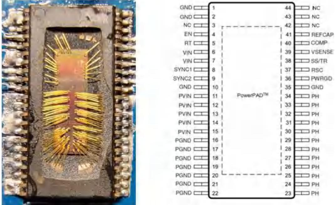
**Figure 3-1. Photograph of Delidded TPS7H4003-SEP [Left] and Pinout Diagram [Right]**
