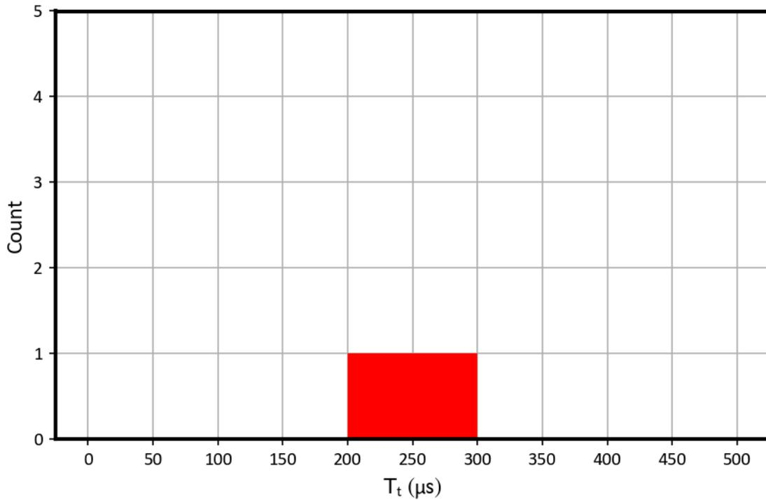
Figure 7-4. Histogram of the Transient Time for  $V_{OUT}$  SETs on Run # 6
