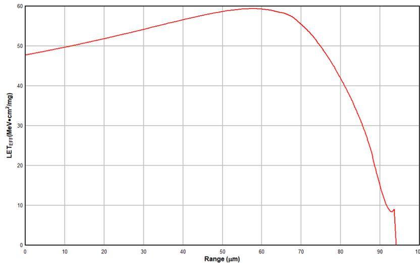
**Figure 5-2. LET<sub>EFF</sub> vs Range for <sup>109</sup>Ag at the Conditions Used for the SEE Test Campaign**
