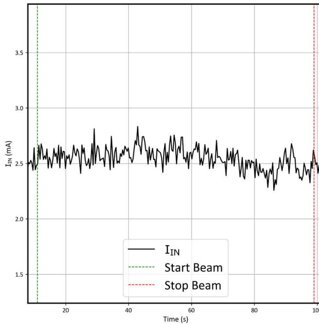
**Figure 7-3. Current vs Time for Run # 7 (Disabled) for the TPS7H4003-SEP at T = 25°C**
