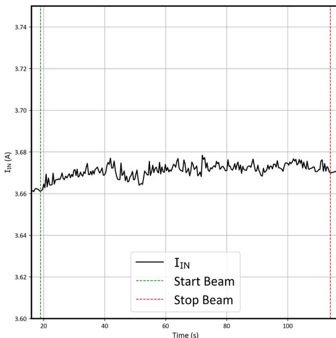
**Figure 7-1. Current vs Time for Run # 1 of the TPS7H4003-SEP at T = 125°C**
