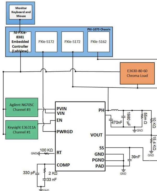
**Figure 6-1. Block Diagram of SEE Test Setup With the TPS7H4003-SEP**
