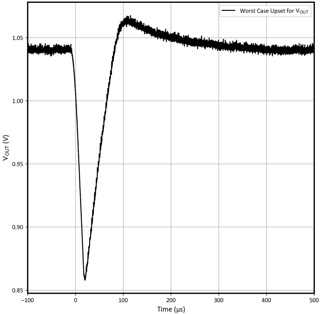
Figure 7-6. Worst Case Positive and Negative Polarity  $V_{OUT\_SET}$  for Run # 6
