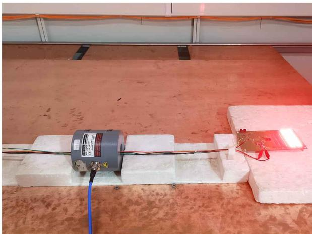
**Figure 3-4. Injection Probe Side of BCI Test**
