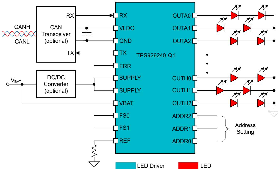
Figure 1-1. TPS929240-Q1 Typical Application Diagram
