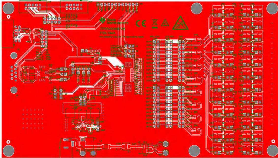
Figure 2-2. TPS929240-Q1 EVM Layout Illustration for BCI Test
