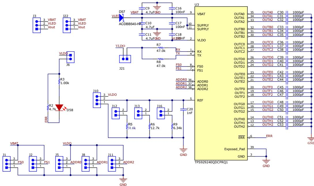
Figure 2-1. TPS929240-Q1 Schematic for PCB Design
