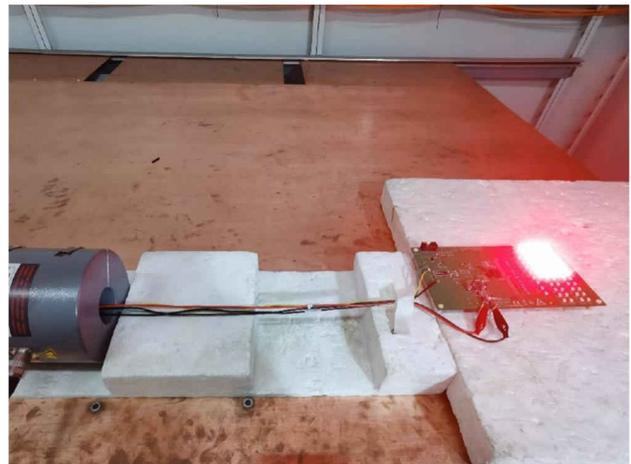
**Figure 3-5. DUT Side of BCI Test**
