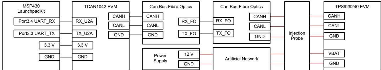
**Figure 3-1. BCI Test Set-up**
