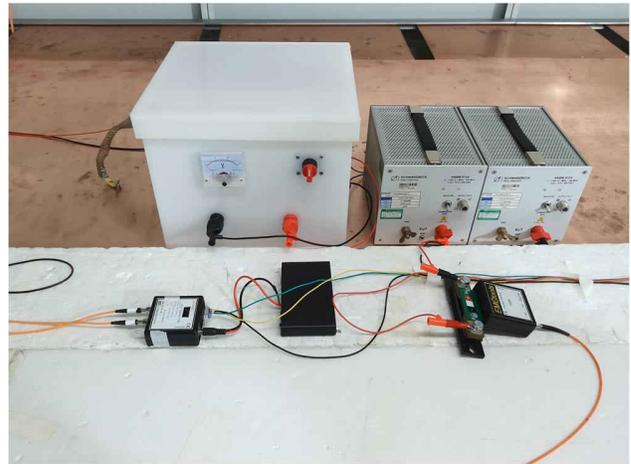
**Figure 3-3. Power Supply Side of BCI Test**
