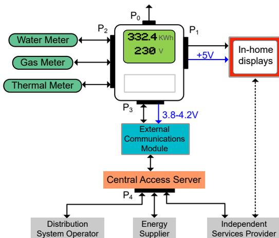
**Figure 1. Illustration of Smart Metering Infrastructure**
