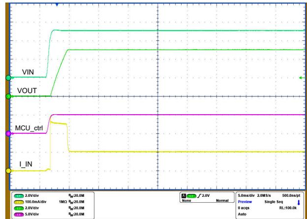
**Figure 7. Successful Startup with a Reset Signal from MCU**
