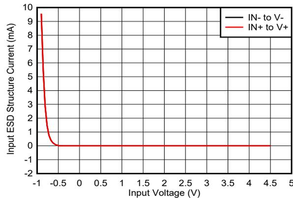
Figure A-15. TLV342/TL342A - Setup 3 - ESD Diode Current for Applied Input Voltage
