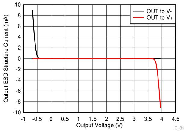
**Figure A-18. OPA310 - Setup 4 - ESD Diode Current for Applied Output Voltage**
