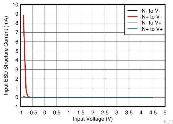
**Figure A-1. OPA310 - Setup 1 - ESD Diode Current for Applied Input Voltage**
