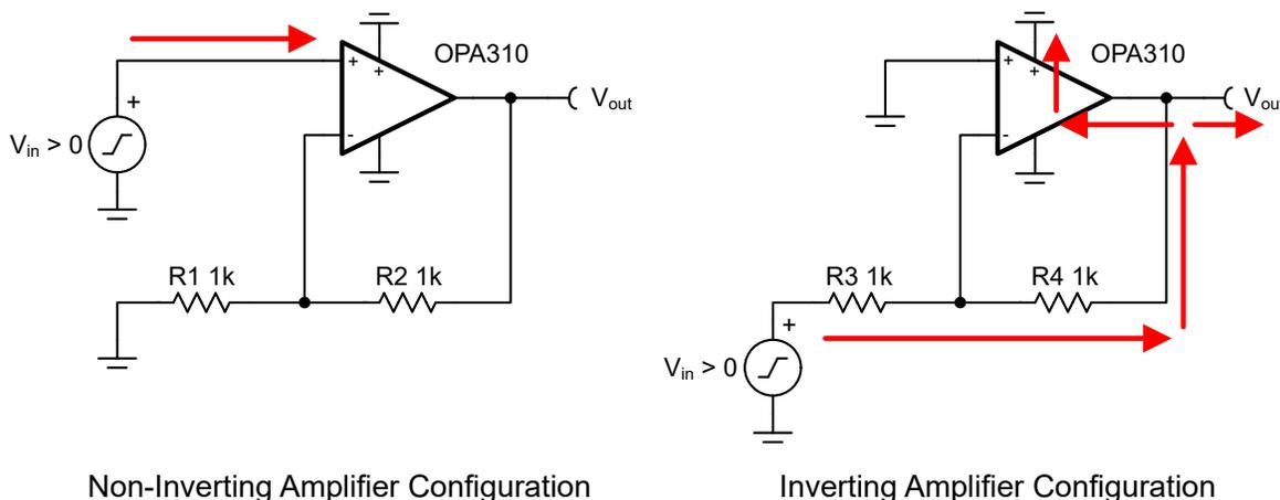
Figure 3-4. Circuit Configuration Can Influence Current Through the ESD Structure
