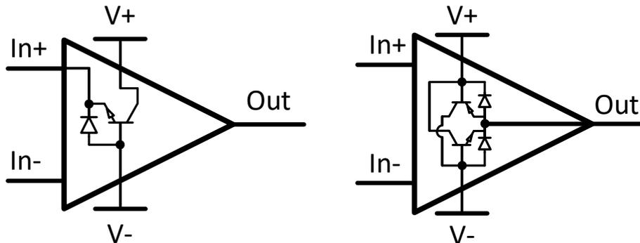
Figure 3-1. Current Paths for IN+ (also present for IN–) and OUT
