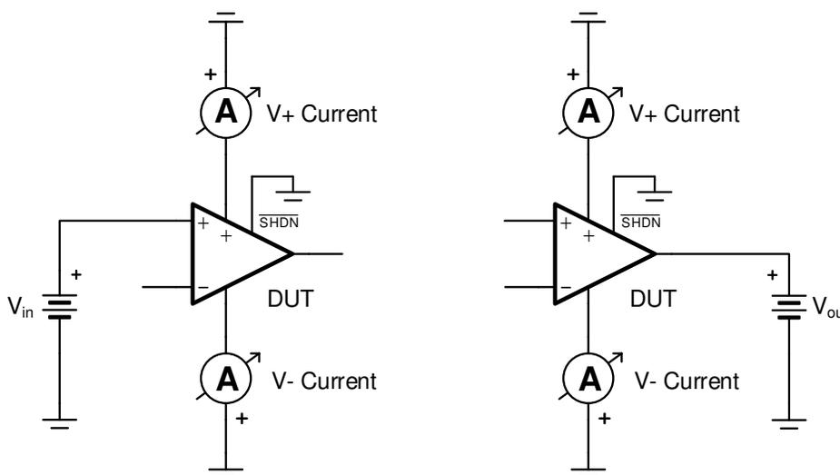
Figure 4-2. Setup 2 - Example Schematic for Testing IN+ and OUT Pins With Grounded Supplies and Shutdown Pin
