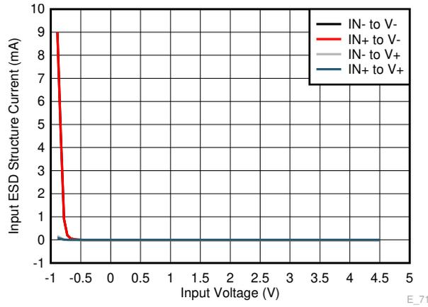
**Figure A-17. OPA310 - Setup 4 - ESD Diode Current for Applied Input Voltage**
