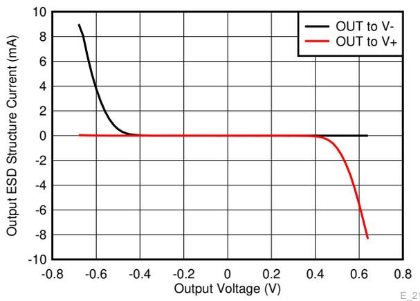
**Figure A-2. OPA310 - Setup 1 - ESD Diode Current for Applied Output Voltage**
