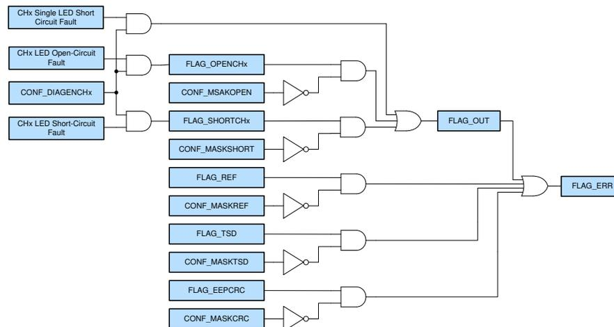
**Figure 5. Diagnostic Enable and Fault Mask**
