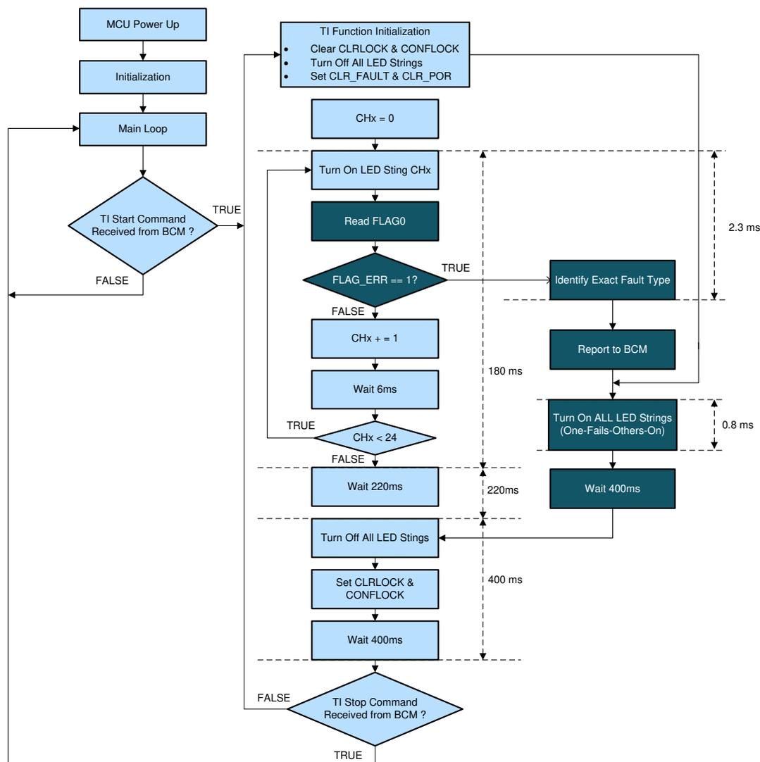
Figure 8. Implement One-Fails-Others-On in Normal State
