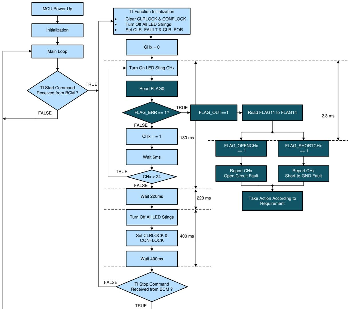
Figure 7. Identify Exact Fault Type in Normal State
