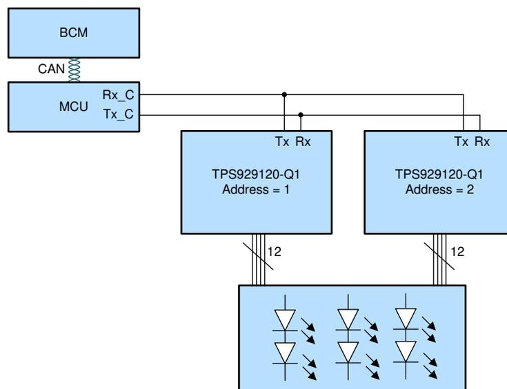
Figure 6. Turn Indicator System Block Diagram in Normal State
