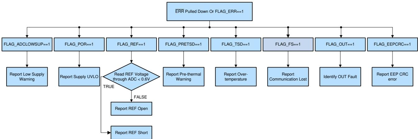
Figure 2. Fault Diagnostic Flow in Normal State
