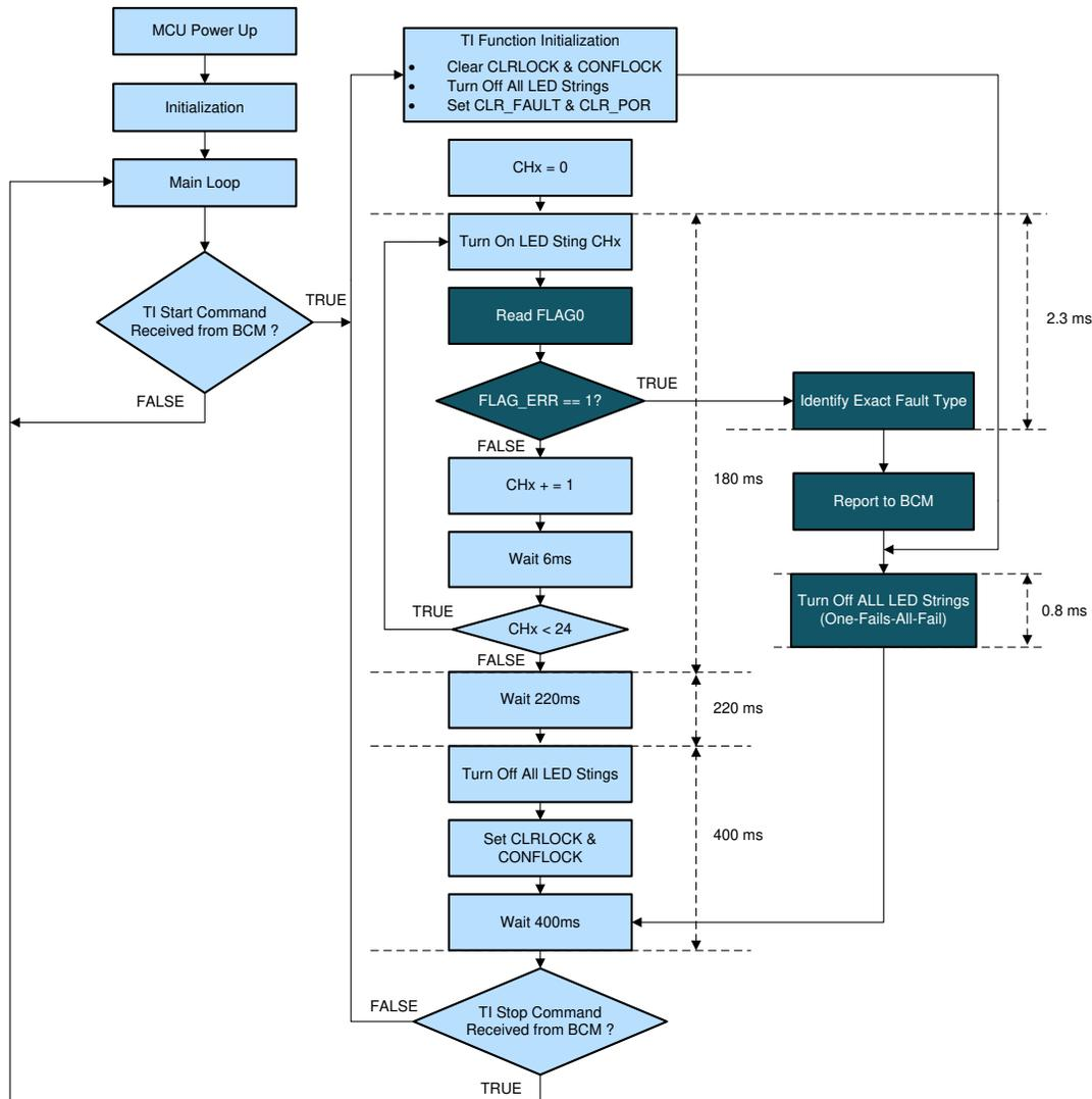
Figure 9. Implement One-Fails-All-Fail in Normal State
