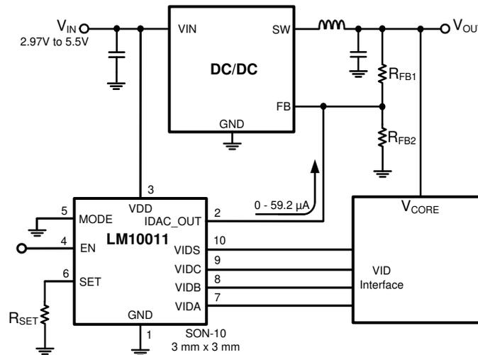
Figure 2-1. Using LM10011 for AVS
