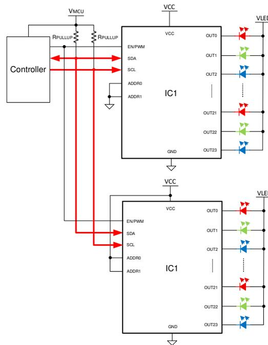
Figure 12. Structure of I<sup>2</sup>C
