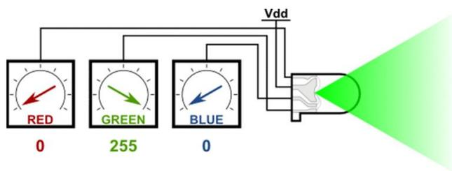
Figure 8. RGB Color Mixing Model
