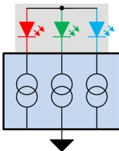
Figure 1. Common Anode LEDs and Current Sink Pair
