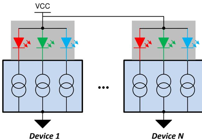
Figure 15. Direct Driving Method
