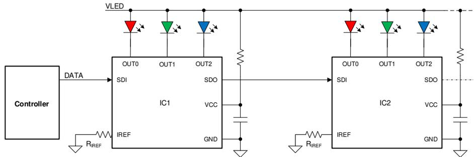
Figure 14. Structure of Single Wire
