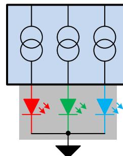
Figure 2. Common Cathode and Current Source Pair
