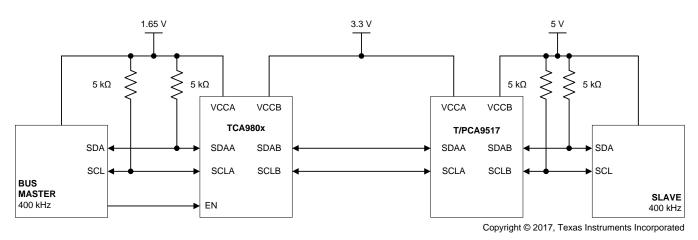
Figure 10. Correct Connection With Other Buffers
