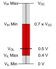
Figure 4. V<sub>oL</sub> Outside of Valid V<sub>IL</sub> Region
