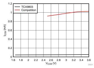
Figure 5. Typical Idle Supply Current ( $I_{CCB}$ ) Across  $V_{CCB}$
