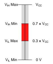
Figure 2. Normal I<sup>2</sup>C Input Thresholds
