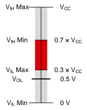
Figure 3.  $V_{OL}$  Within Valid  $V_{IL}$  Region
