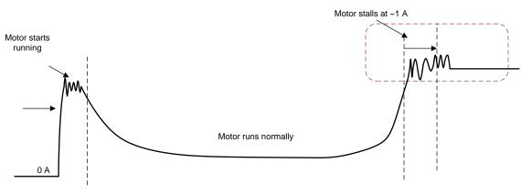
Figure 6. Motor-Current Profile
