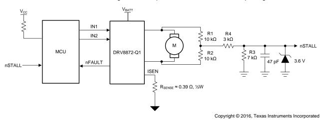
Figure 4. Typical Stall-Detection Circuit
