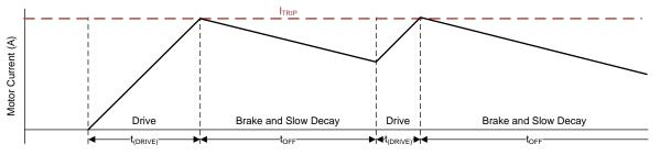
Figure 3. Internal Current-Chopping Timing Diagram
