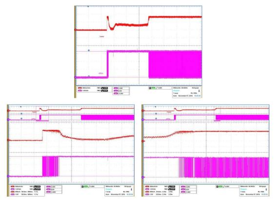
Figure 8. Reverse Direction Motor Stalling
