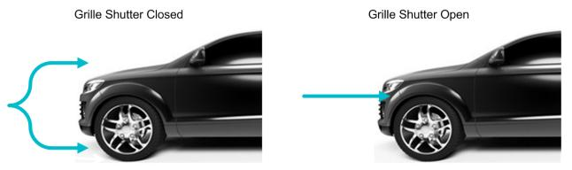
Figure 1. Air Flow With Grille Shutter Open and Closed
