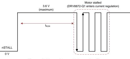
Figure 5. Motor Phase-Voltage Profile
