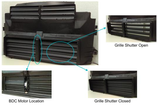
Figure 2. Active Grille Shutter Operation
