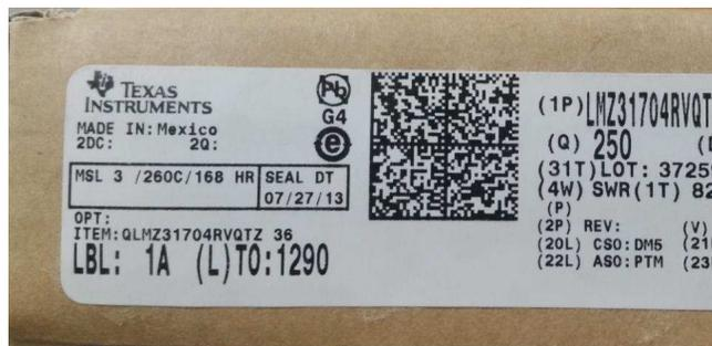
**Figure 2. MSL Rating and Peak Reflow Labeling on Box**
