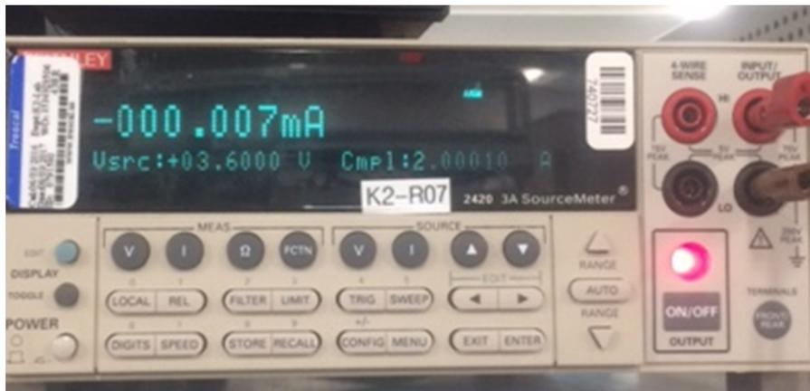
Figure 6. Reduced Leakage Current Confirmed with Keithley Sourcemeter
