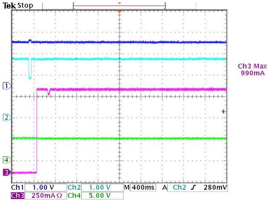
Figure 9. TPS25810 and TPS2544 (DCP Auto Mode) Test With Galaxy S6, With Type C-to-B Dongle Connected to Host Then Plug In Device
