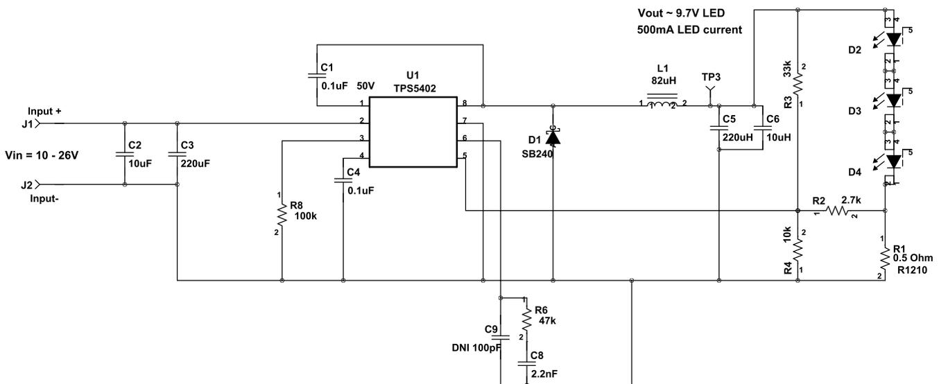
Figure 11. Simple LED Driver Implementation using TPS5402
