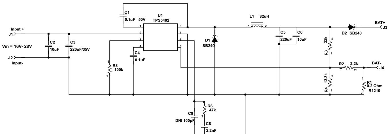
Figure 1. Linear Current Tapering Charger Using TPS5402
