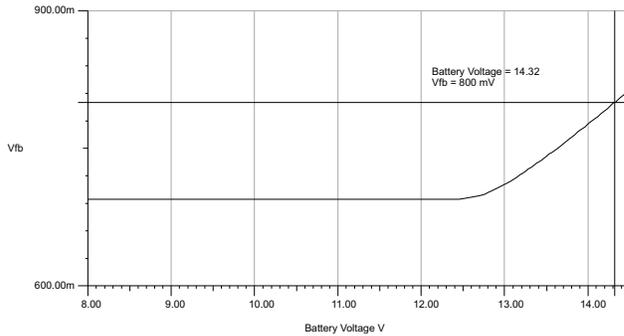
Figure 7. Feedback Voltage vs. Battery Voltage
