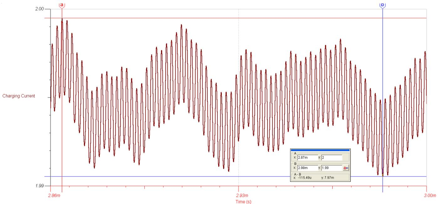
The current ripple during the CC Mode is found to be around 8mA. The ripple frequency noticed is that of the switching frequency.
