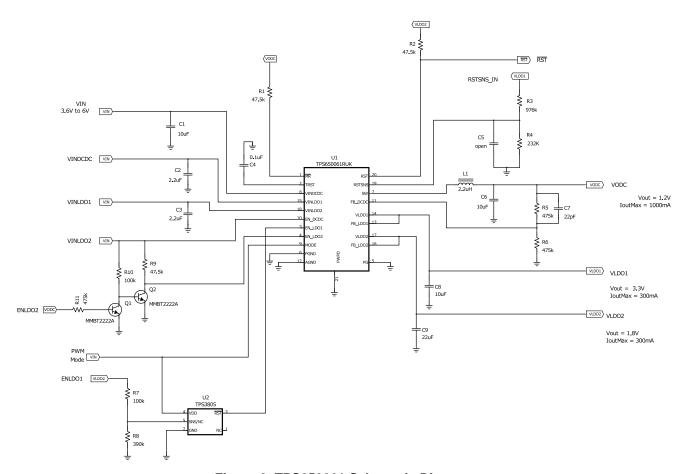
Figure 2. TPS650061 Schematic Diagram
