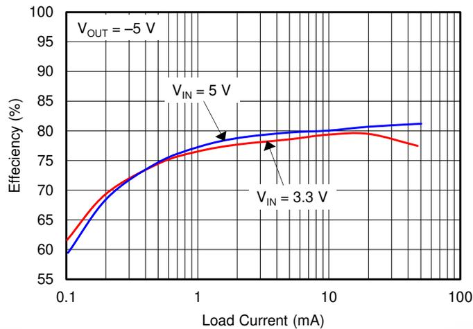
Figure 5-2. Efficiency versus Load Current with  $V_{OUT} = -5\text{ V}$
