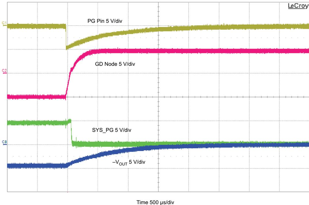
**Figure 2-7. PG Pin Level Shifter on Shutdown**
