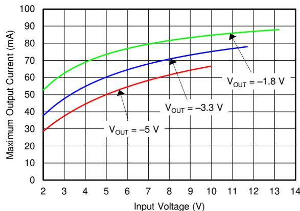
**Figure 1-4. Maximum Output Current versus Input Voltage**
