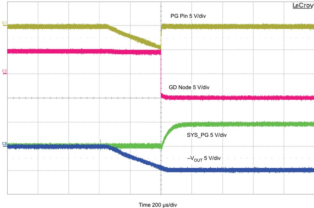
**Figure 2-6. PG Pin Level Shifter on Startup**
