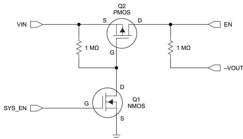
$V_{OUT}$  is the negative output voltage of the inverting buck-boost converter
