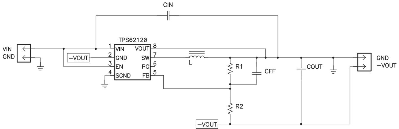
**Figure 1-2. TPS62120 Inverting Buck-Boost Topology**
