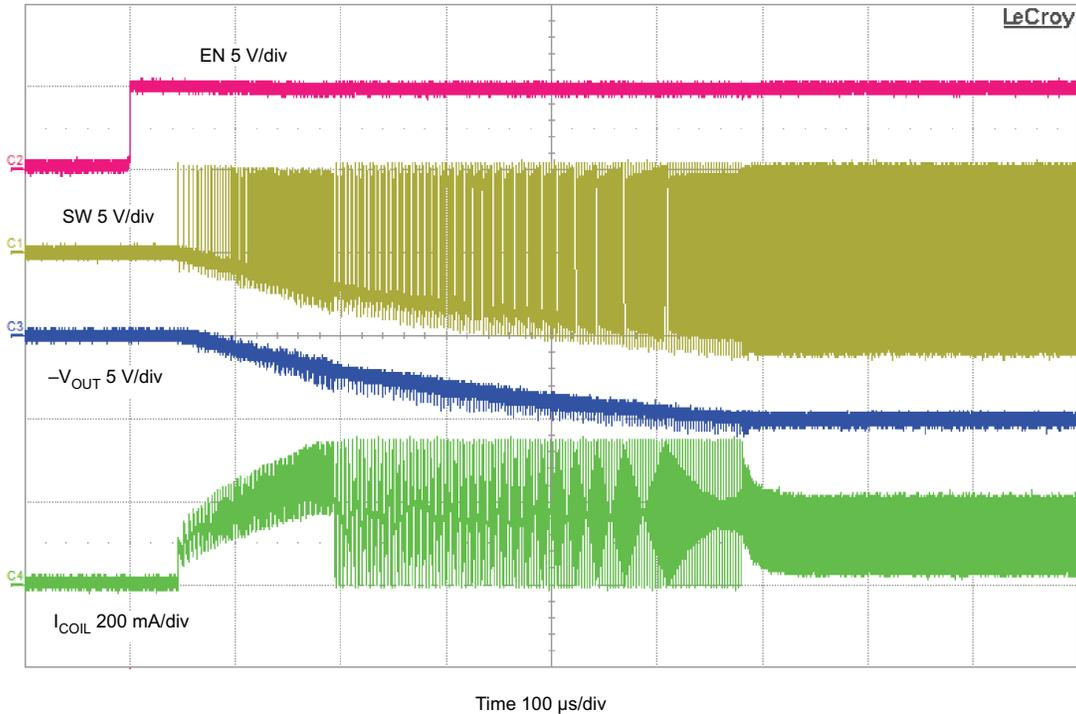
Figure 3-1. Startup Behavior in the Inverting Configuration
