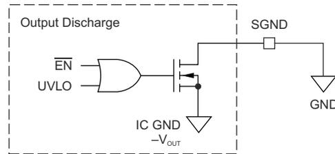
Figure 2-4. SGND Internal Circuit
