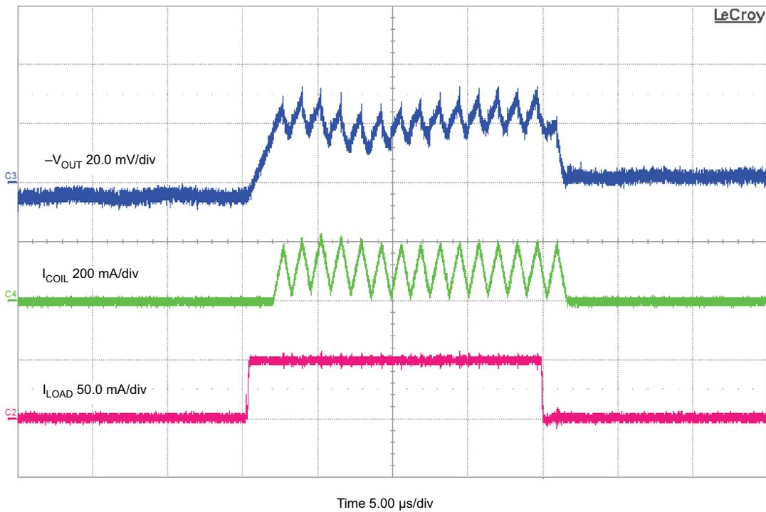
Figure 5-5. Load Transient Response 0 mA to 50 mA with  $V_{IN} = 5 V$
