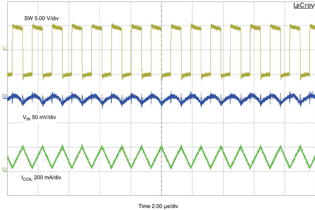
**Figure 5-6. Input Voltage Ripple,  $V_{IN} = 5$  V and  $I_{OUT} = 50$  mA**
