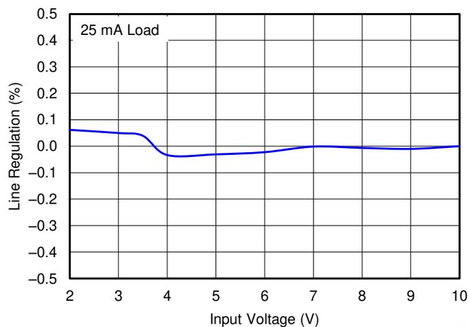
Figure 5-3. Line Regulation with  $V_{OUT} = -5\text{ V}$  and 25-mA Load
