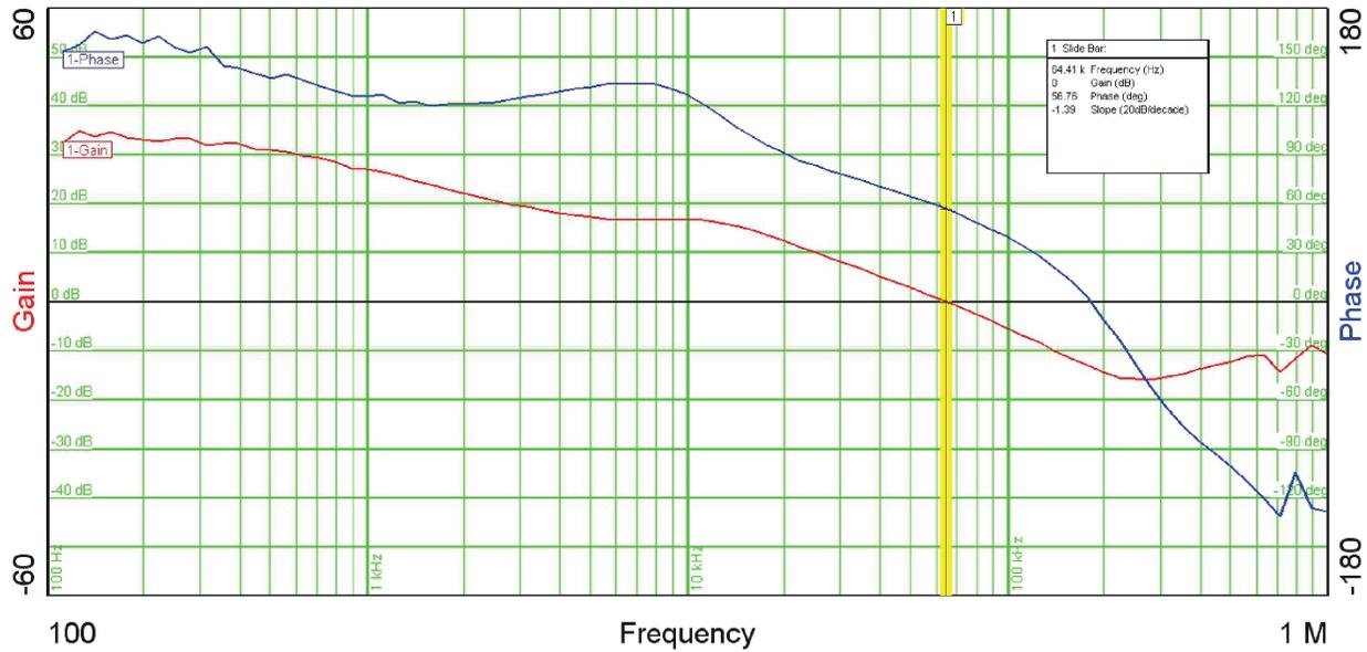
Figure 4-2. Bode Plot at 5-V  $V_{IN}$  and 50-mA Load
