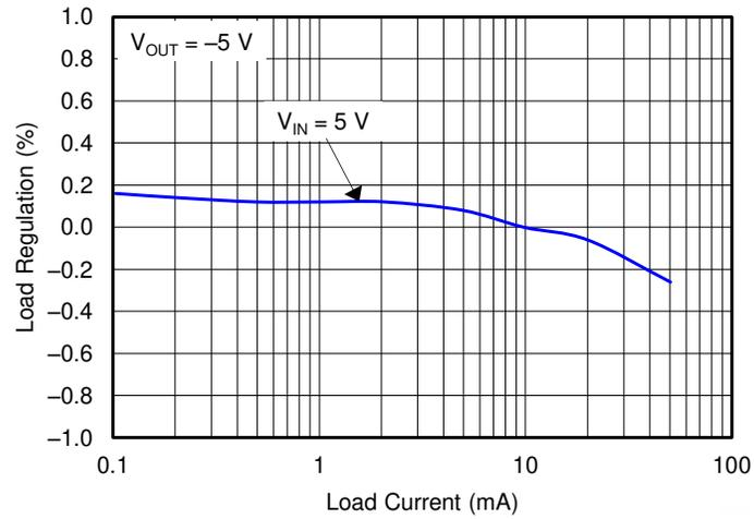
Figure 5-4. Load Regulation with  $V_{OUT} = -5 V$
