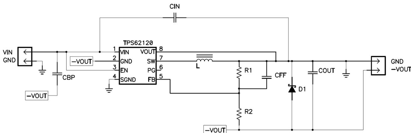
Figure 4-1. If Installing CBP, Installing Schottky D1 is Required
