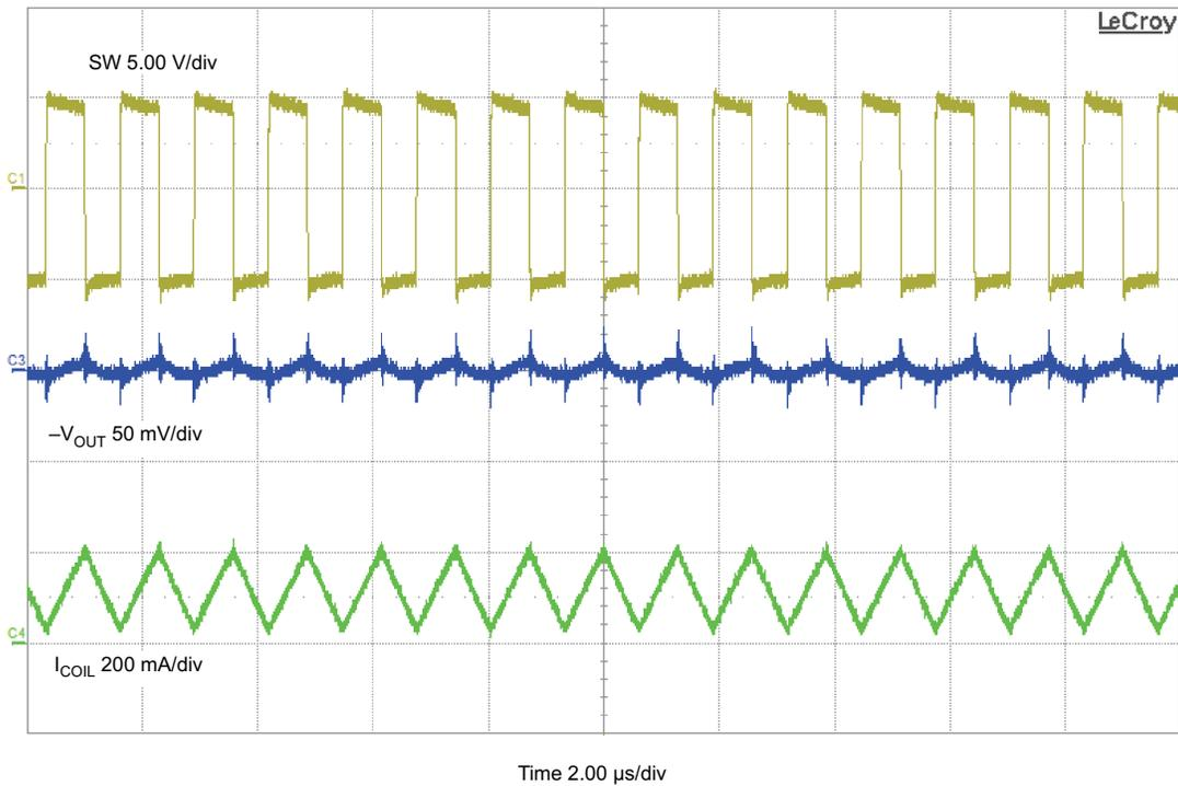
**Figure 5-7. Output Voltage Ripple,  $V_{IN} = 5$  V and  $I_{OUT} = 50$  mA**
