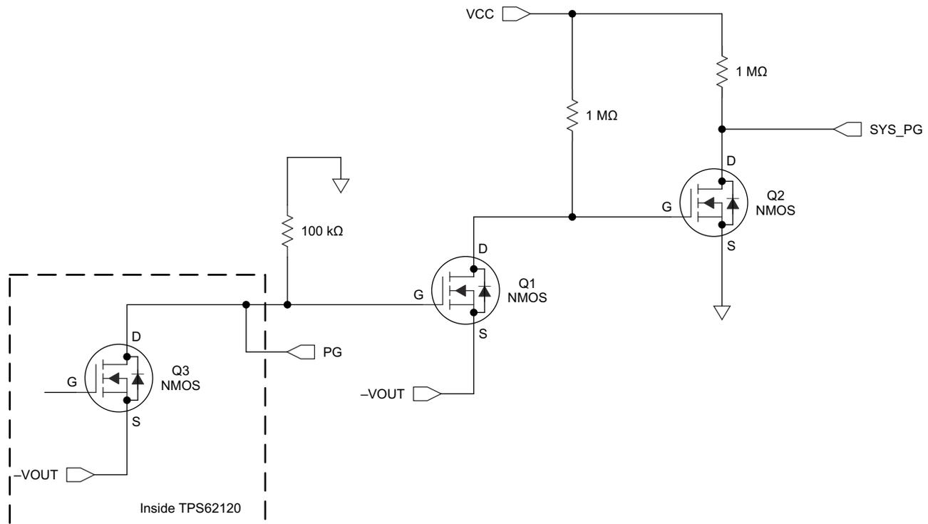
Figure 2-5. PG Pin Level Shifter
