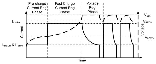
Figure 1. Algorithm for Pulse Current Charging
