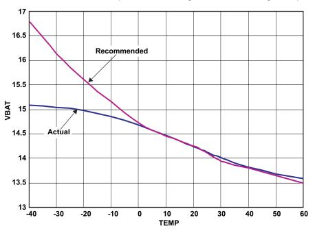
Figure 3. Battery Voltage vs Temperature for a 6-cell, Sealed, Lead-Acid Battery
